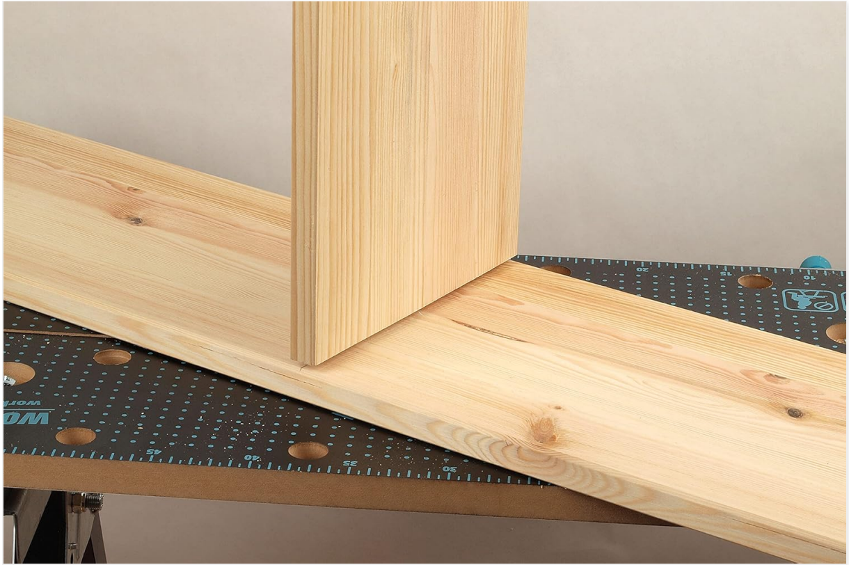
Figure 5: An example of a T-butt joint, where one board is joined perpendicularly to the face of another using dowel pins. For T-butt connections, drill holes into the end grain of one board and into the face of the other. Ensure the holes align perfectly before pressing the pieces together. Clamp the joint until the glue dries.
