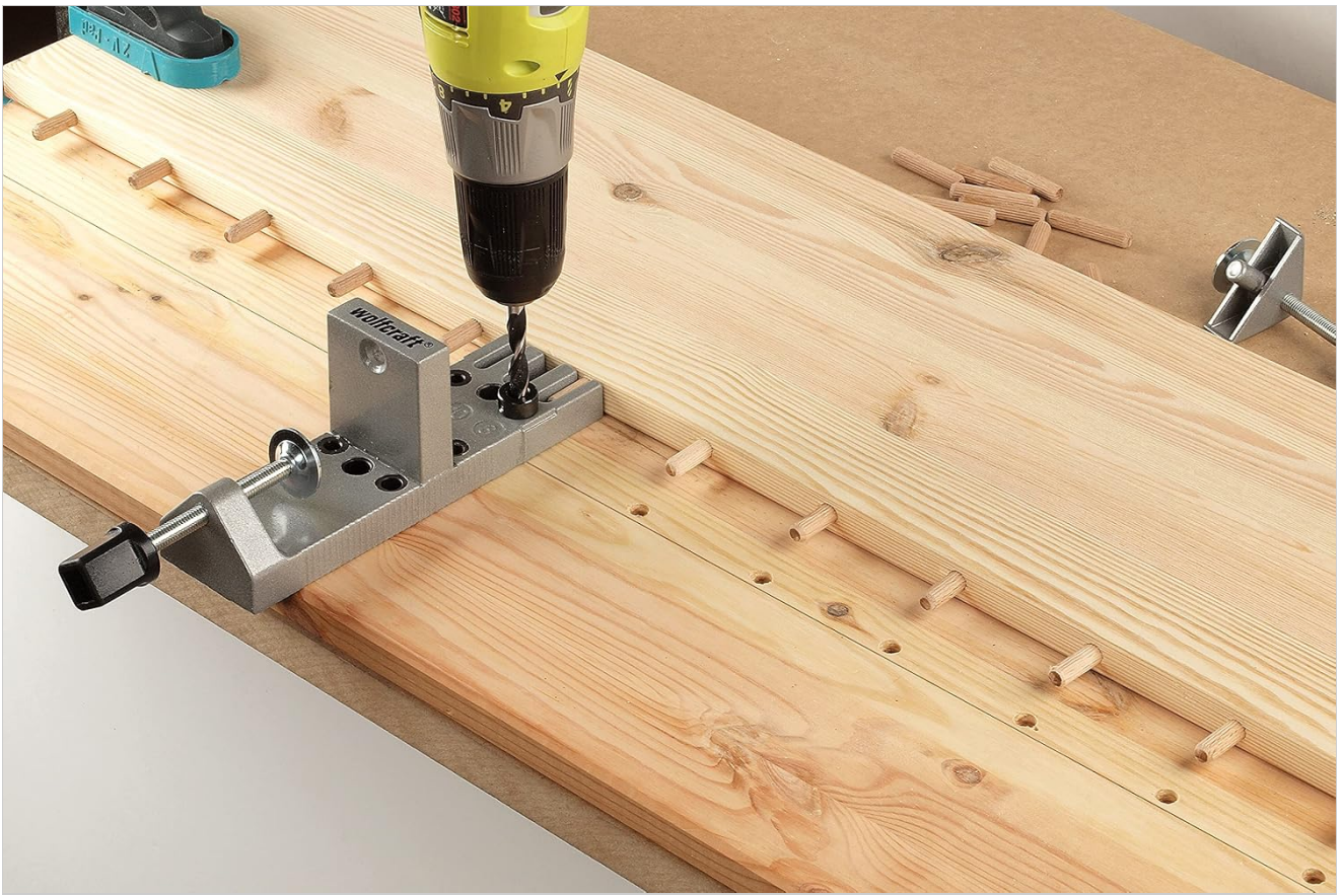
Image 5.1: A power drill being used with the Wolfcraft dowelling jig to create precise holes for dowels.
