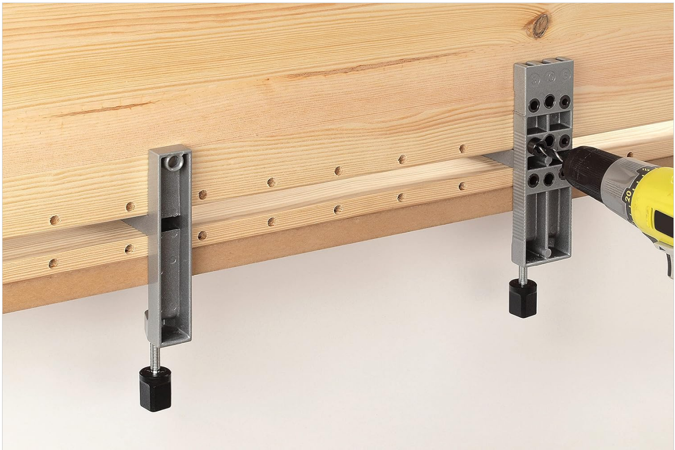
Image 4.1: The dowelling jig securely clamped to a wooden board, ready for drilling.
