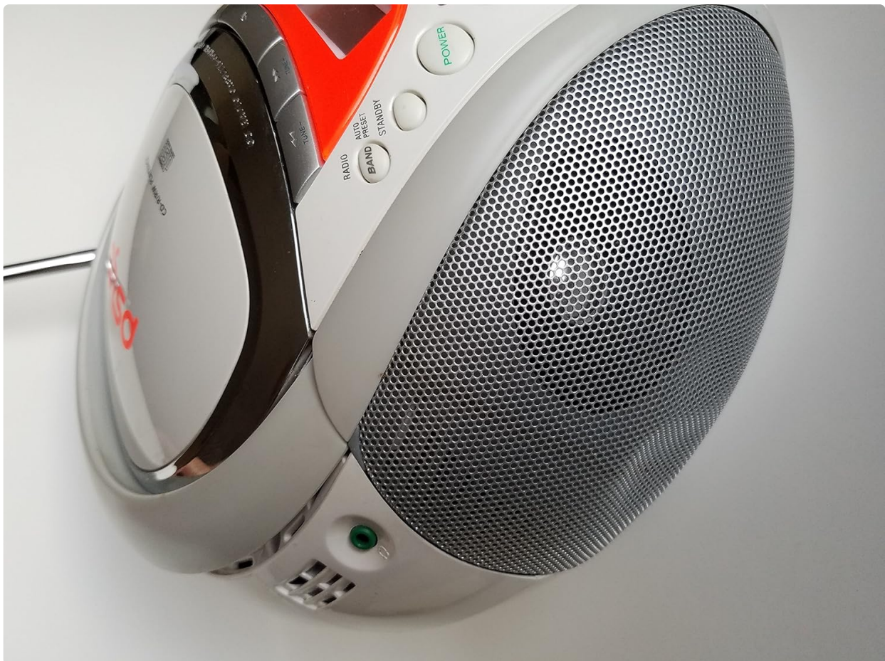
Figure 4.2: Side view of the unit, highlighting the headphone jack for private listening.
