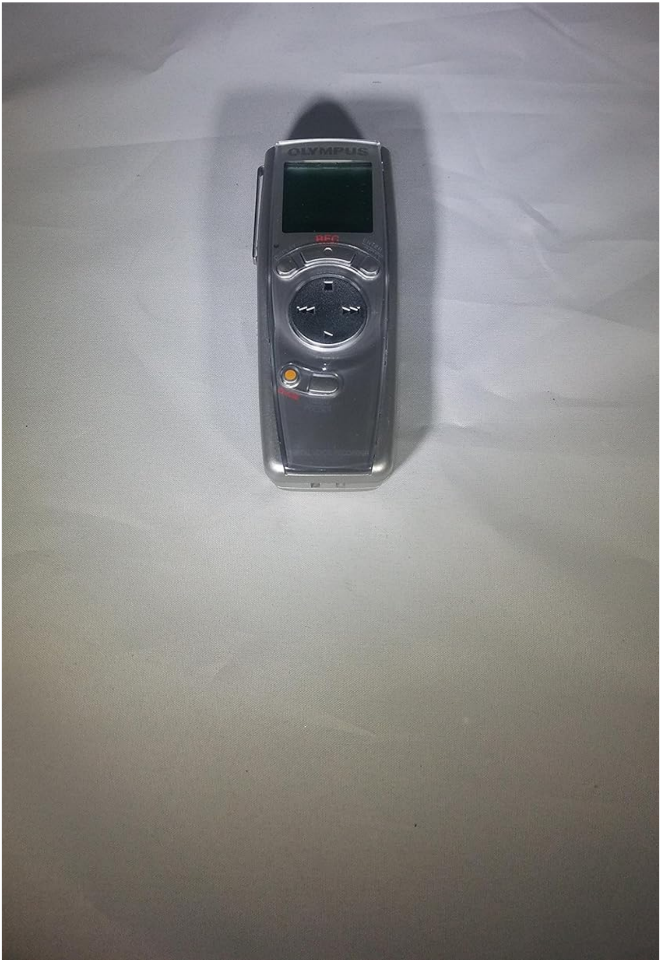
Figure 3.1: Front View of VN-480PC. This image displays the front of the Olympus VN-480PC digital voice recorder, showing the LCD screen, navigation thumb-pad, and recording/playback buttons. The device is silver-colored with a dark screen and black controls.
