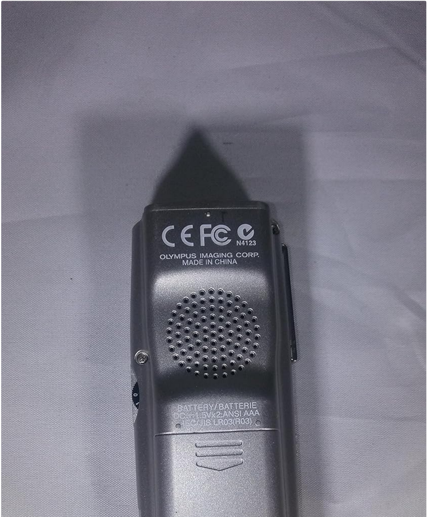
Figure 3.2: Rear View of VN-480PC. This image shows the back of the Olympus VN-480PC digital voice recorder, highlighting the built-in speaker grille, battery compartment cover, and regulatory markings. The device is silver with a textured speaker area.
