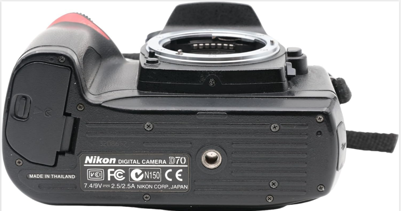
Figure 2.4: Bottom View. This image displays the bottom of the Nikon D70, showing the battery compartment cover and the tripod socket.
