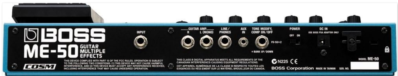
Figure 2: Rear panel of the Boss ME-50, showing input, output, and power connections.
