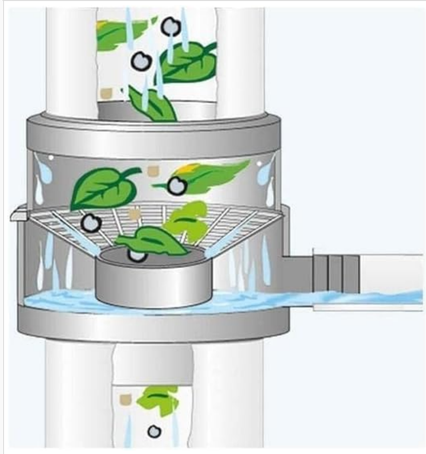
Figure 2: An illustrative diagram showing the internal mechanism of the filter header. Rainwater flows down the downpipe, passes through an internal sieve that deflects leaves and debris, and then is diverted through the side outlet into a rain barrel. Excess water continues down the main downpipe, preventing barrel overflow.
