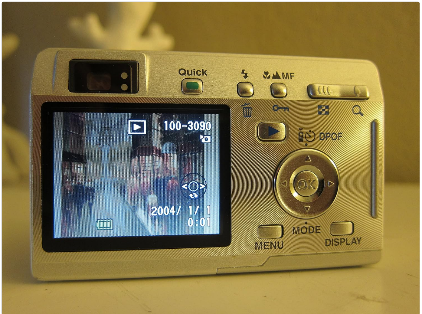
Figure 5: Rear view of the camera with the LCD screen displaying an image in playback mode, showing navigation controls.
