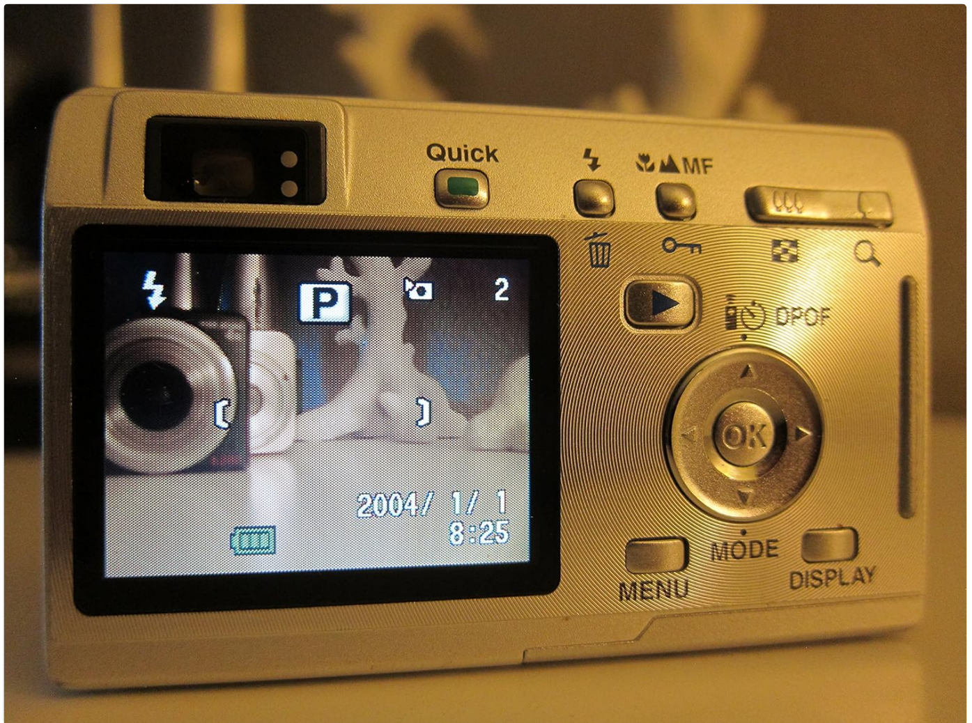
Figure 4: Rear view of the camera displaying the LCD screen in shooting mode, with various controls visible for mode selection and navigation.
