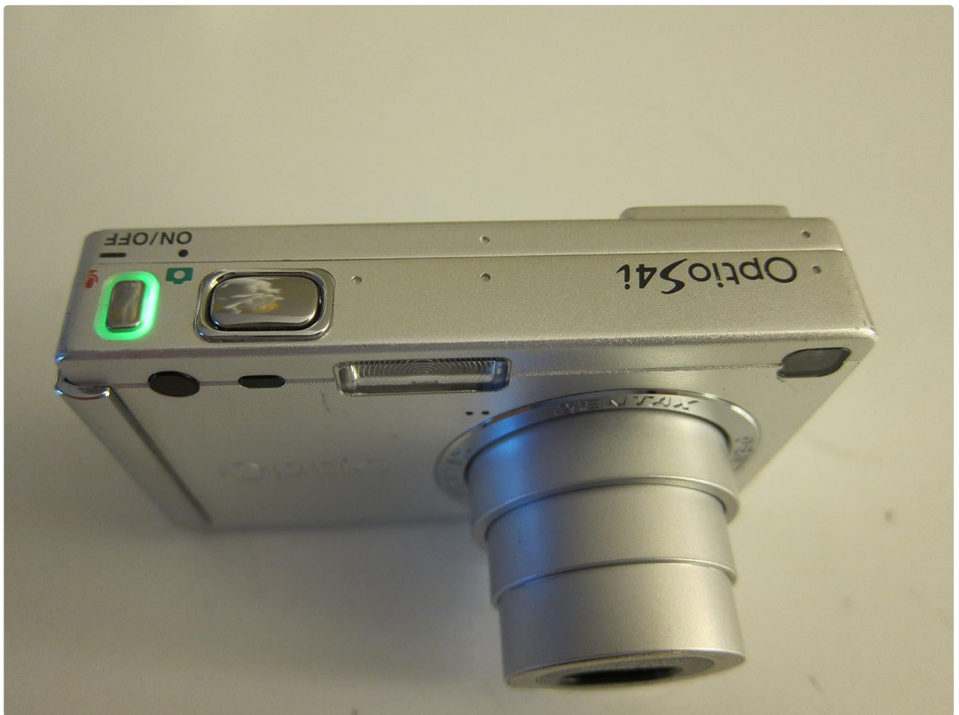
Figure 2: Top view of the camera, highlighting the ON/OFF button. Press this button to power the camera on or off.
