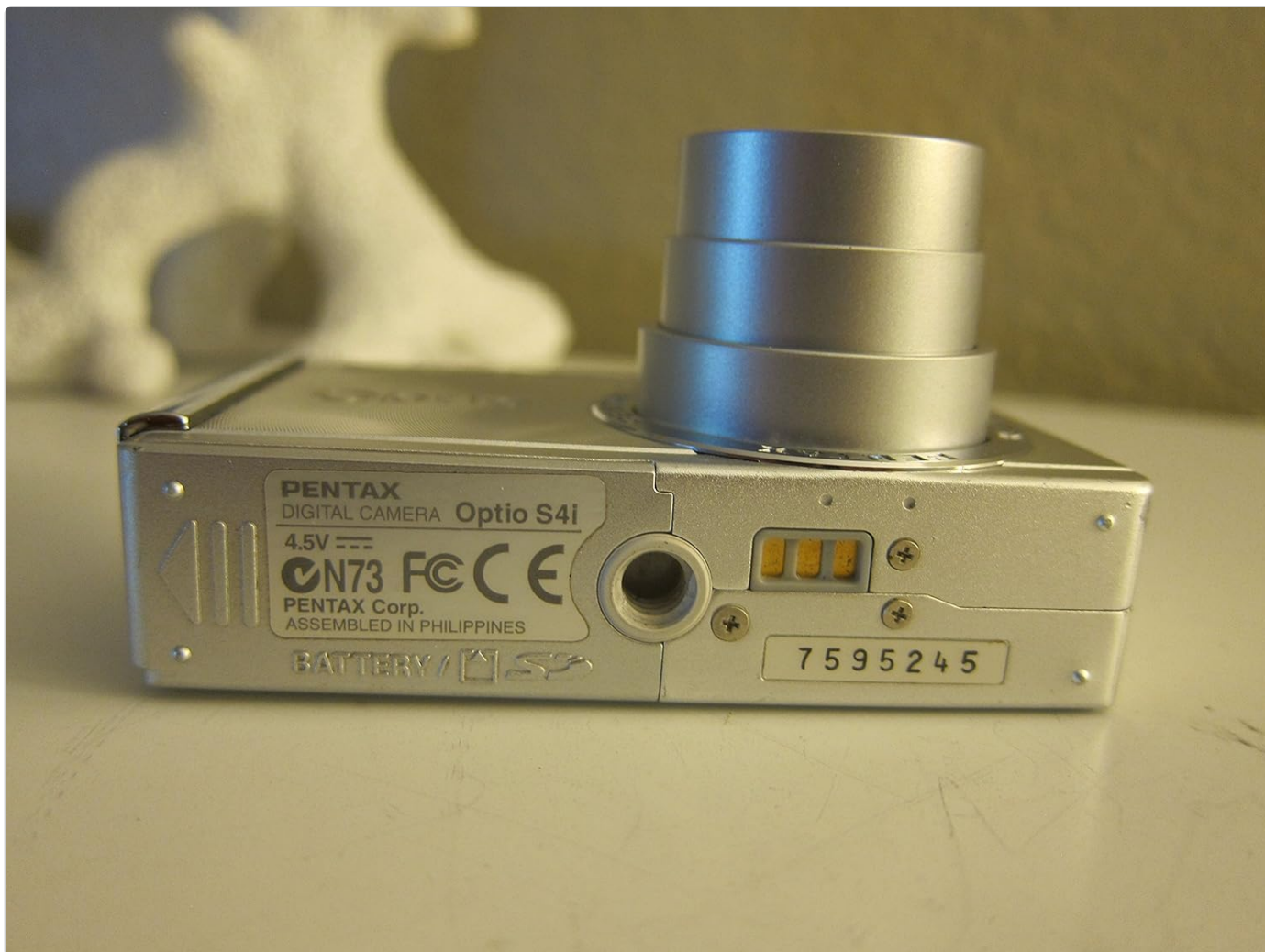
Figure 1: Bottom view of the camera, illustrating the battery and SD card compartment. This is where the Lithium-Ion battery is inserted and secured.
