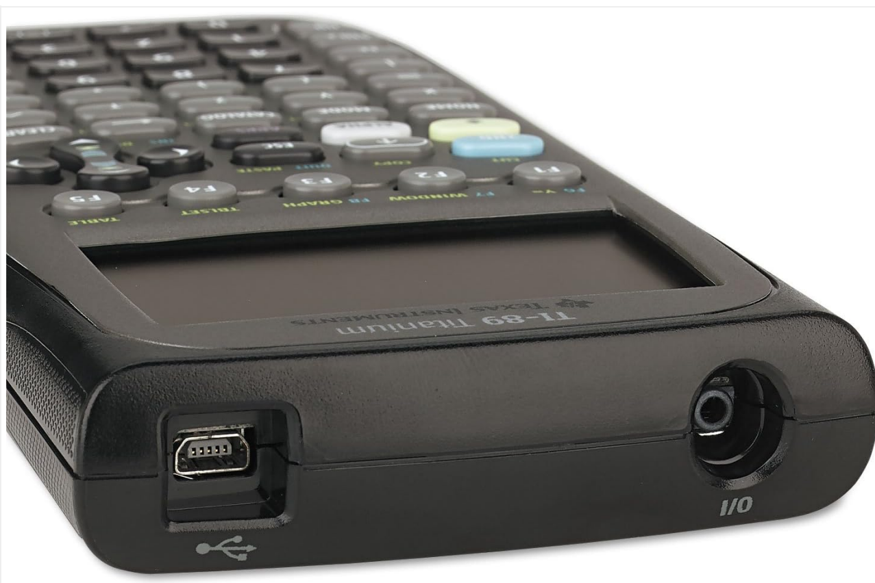
Image: A close-up view of the TI-89 Titanium's USB port and I/O port, located on the top edge of the calculator.
