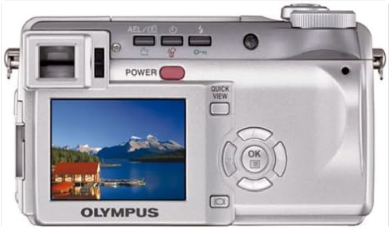
Figure 4.1: The rear panel of the camera, highlighting the LCD screen, power button, and navigation controls for menu access and photo review.
