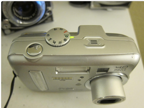
Top view of the camera, showing the mode dial and shutter button.
