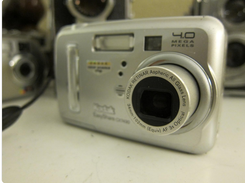
Front view of the camera with the 3x optical zoom lens extended.
