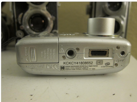
Bottom view of the camera, displaying the battery/memory card compartment and USB port.
