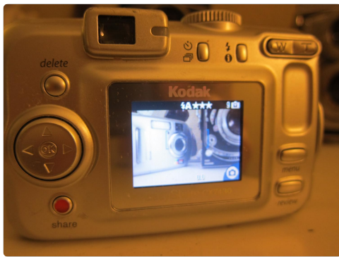
Back view of the camera, showing the 1.6-inch LCD screen and control buttons.
