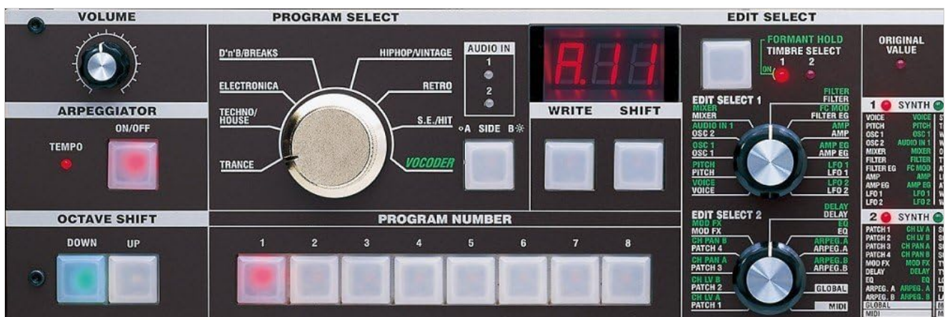
Figure 3.2: Close-up of the microKORG's central control panel, showing the Program Select rotary switch, the digital display, and the Edit Select 1 and 2 knobs with their corresponding parameter lists.
