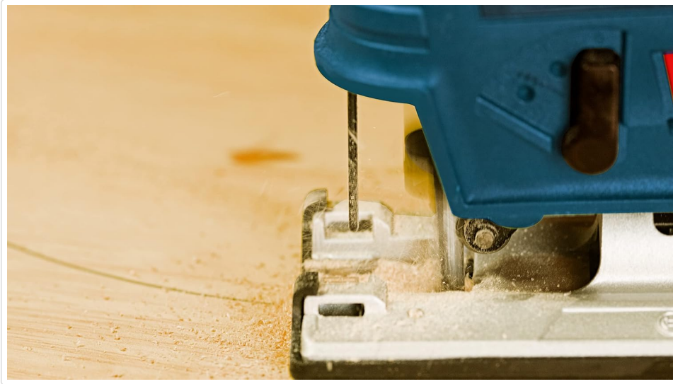
Image: A T-shank jigsaw blade being inserted into the blade clamp of a jigsaw, demonstrating the installation process.
