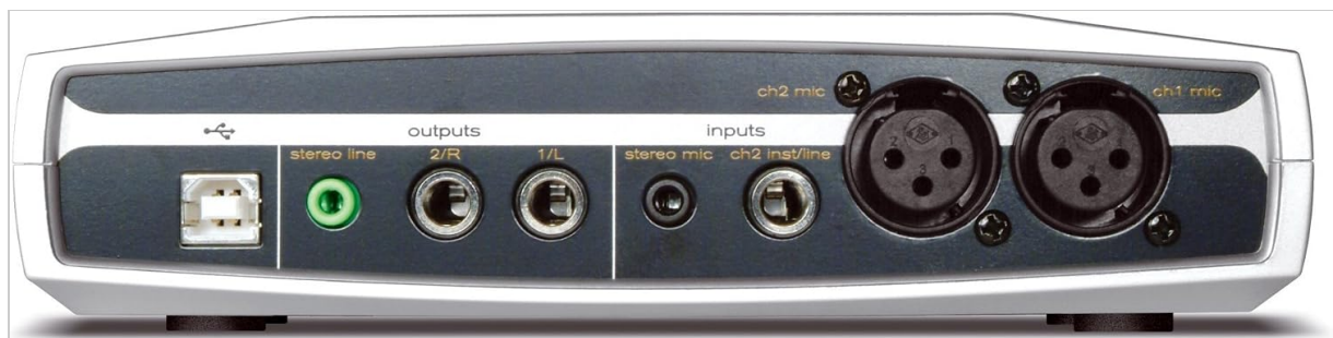
Figure 2: Rear panel of the M-Audio MobilePre USB, displaying USB port, stereo line output, 1/4" TRS outputs, stereo mic input, and XLR microphone inputs.
