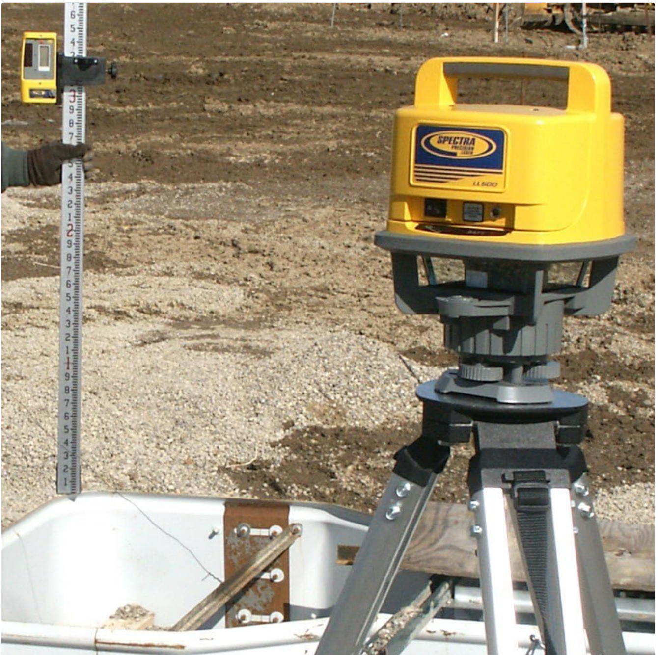
Figure 4: HL700 Receiver mounted on a grade rod in use.
