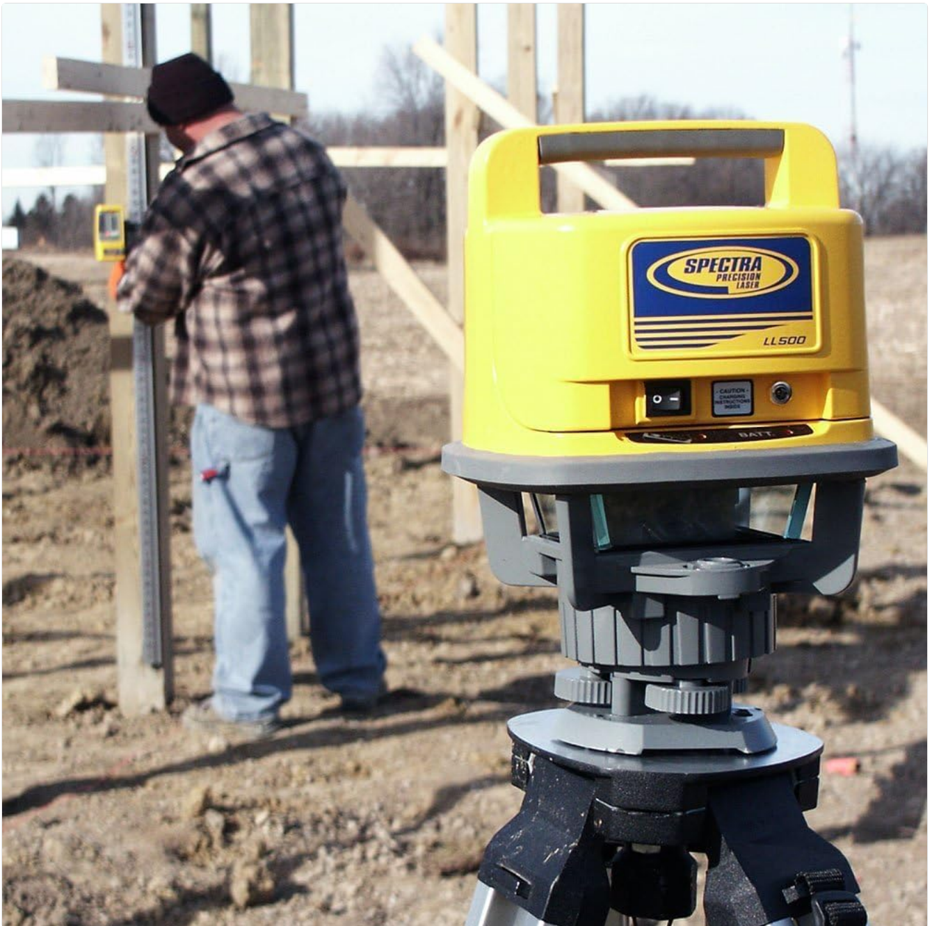
Figure 5: LL500 Laser Level in use for general site leveling.
