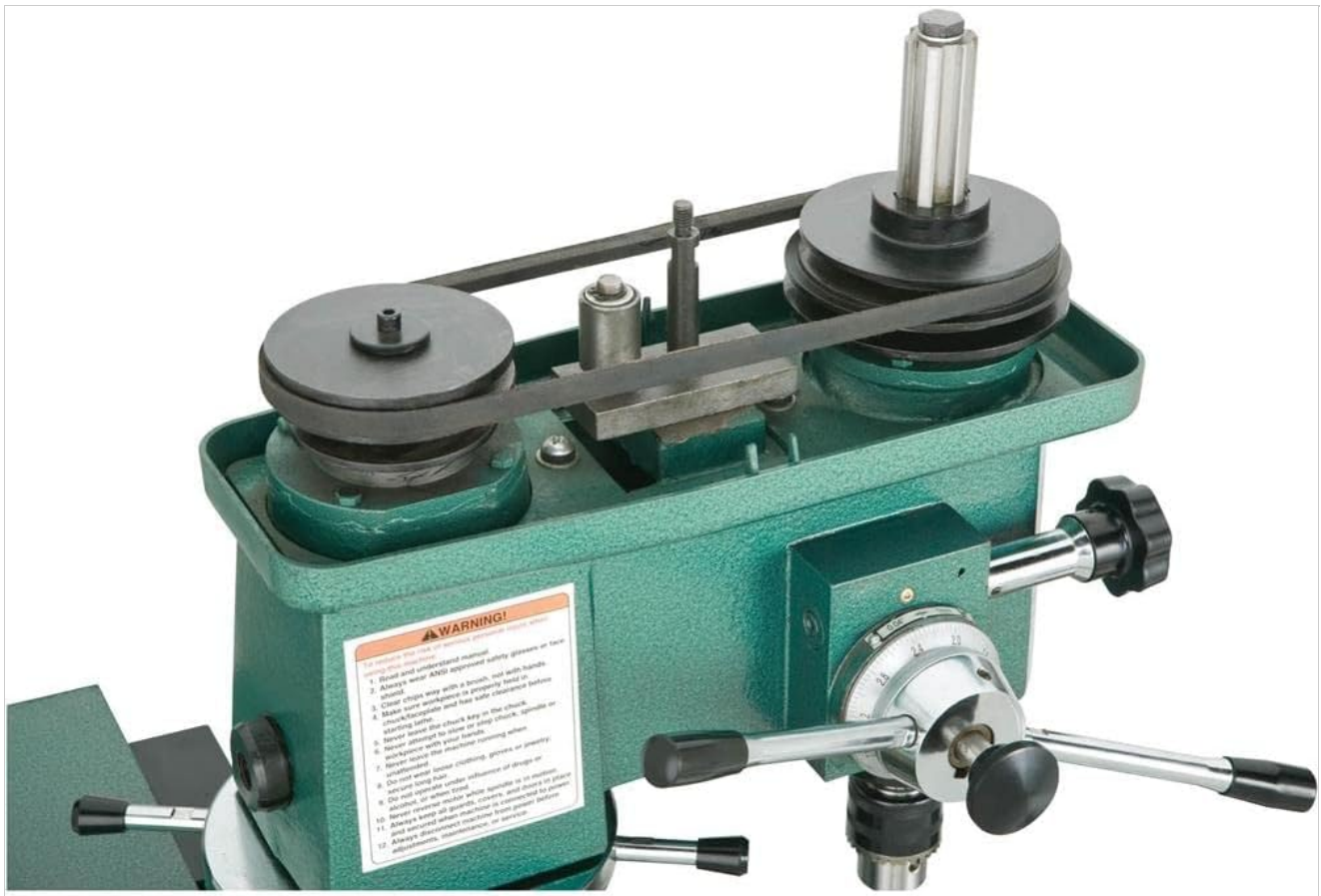
Figure 4: Top view of the milling head, illustrating the belt drive system for changing spindle speeds.
