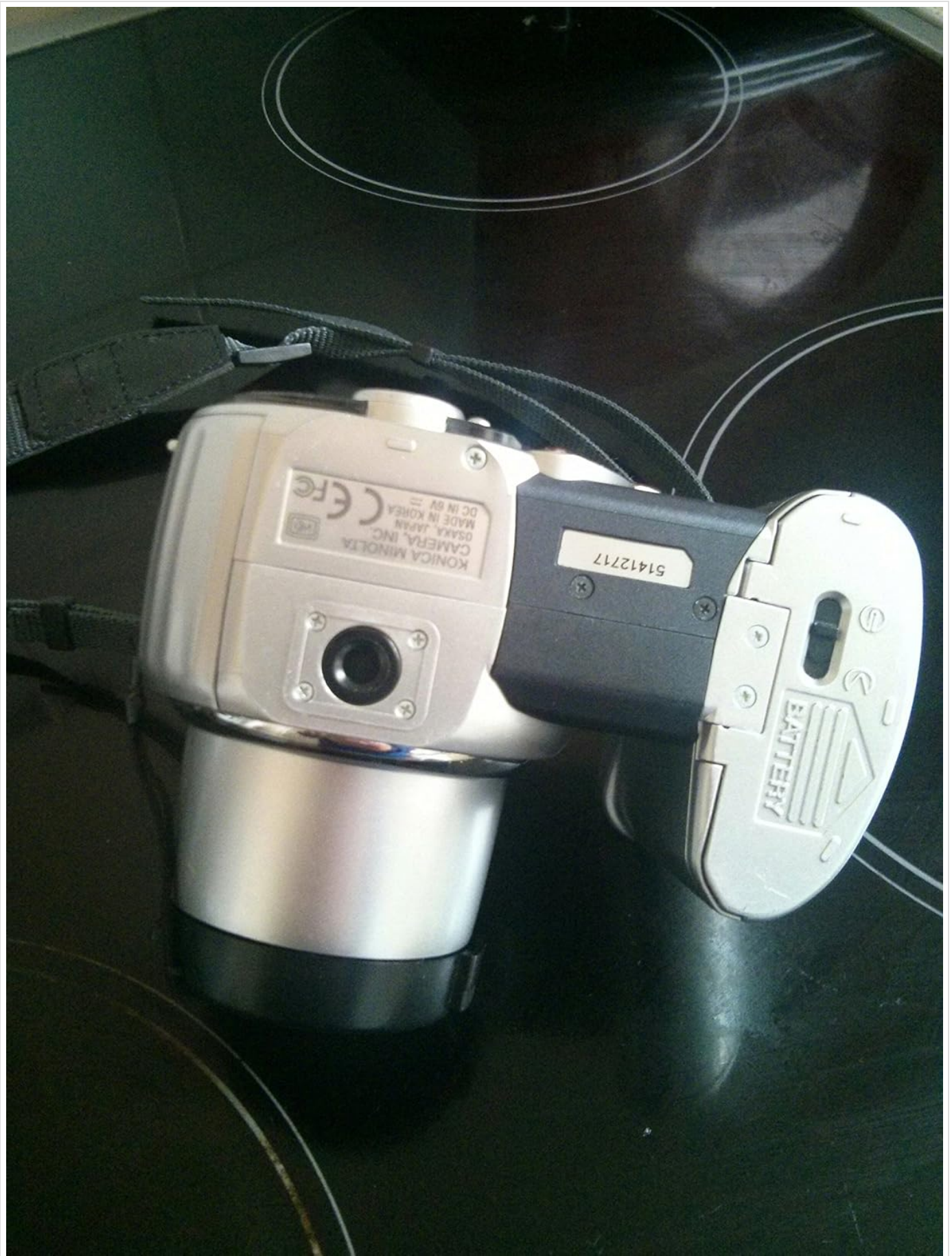
Figure 1: Bottom view of the Minolta Dimage Z1, highlighting the battery compartment and tripod mount.
