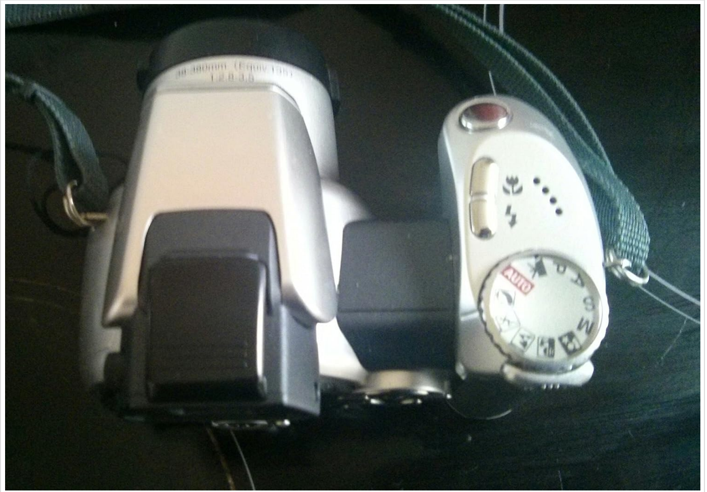
Figure 3: Top view of the Minolta Dimage Z1, illustrating the main controls including the mode dial.
