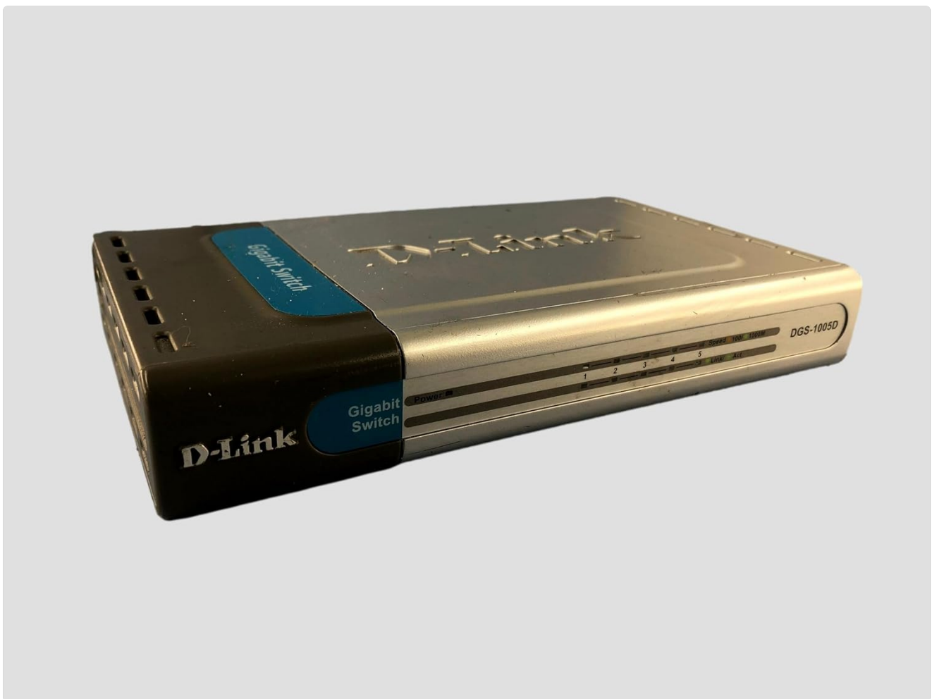
Figure 1: Front view of the D-Link DGS-1005D 5-Port Gigabit Switch, showing the D-Link logo, "Gigabit Switch" label, and five LED indicators for ports 1-5.
