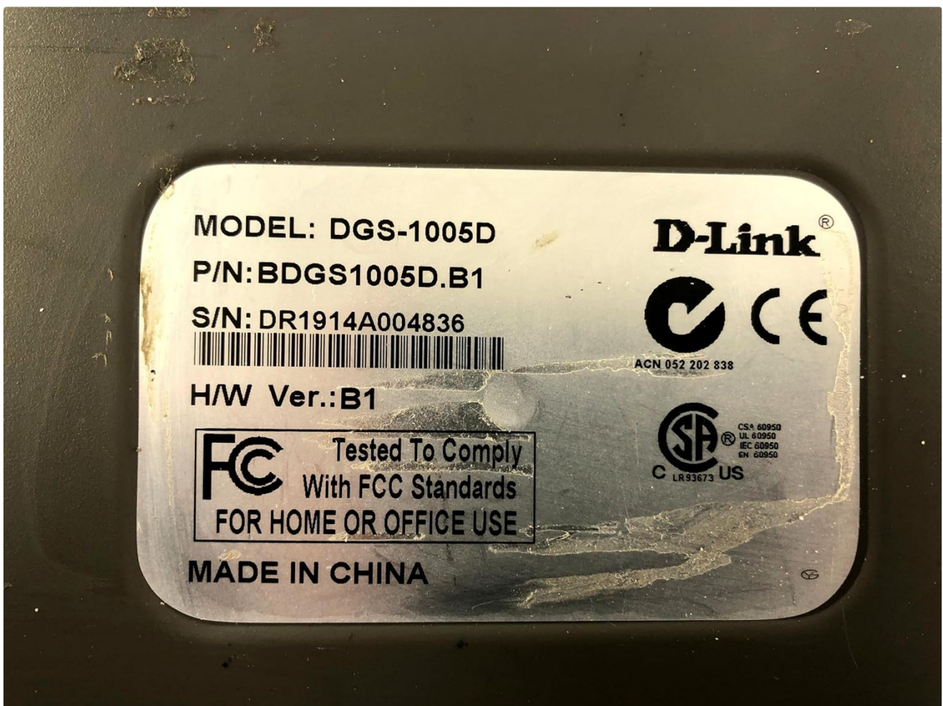
Figure 3: Bottom label of the D-Link DGS-1005D switch, displaying the model number (DGS-1005D), part number (BDGS1005D.B1), serial number (DR1914A004836), hardware version (B1), and regulatory compliance marks (FCC, CE, CSA, UL).
