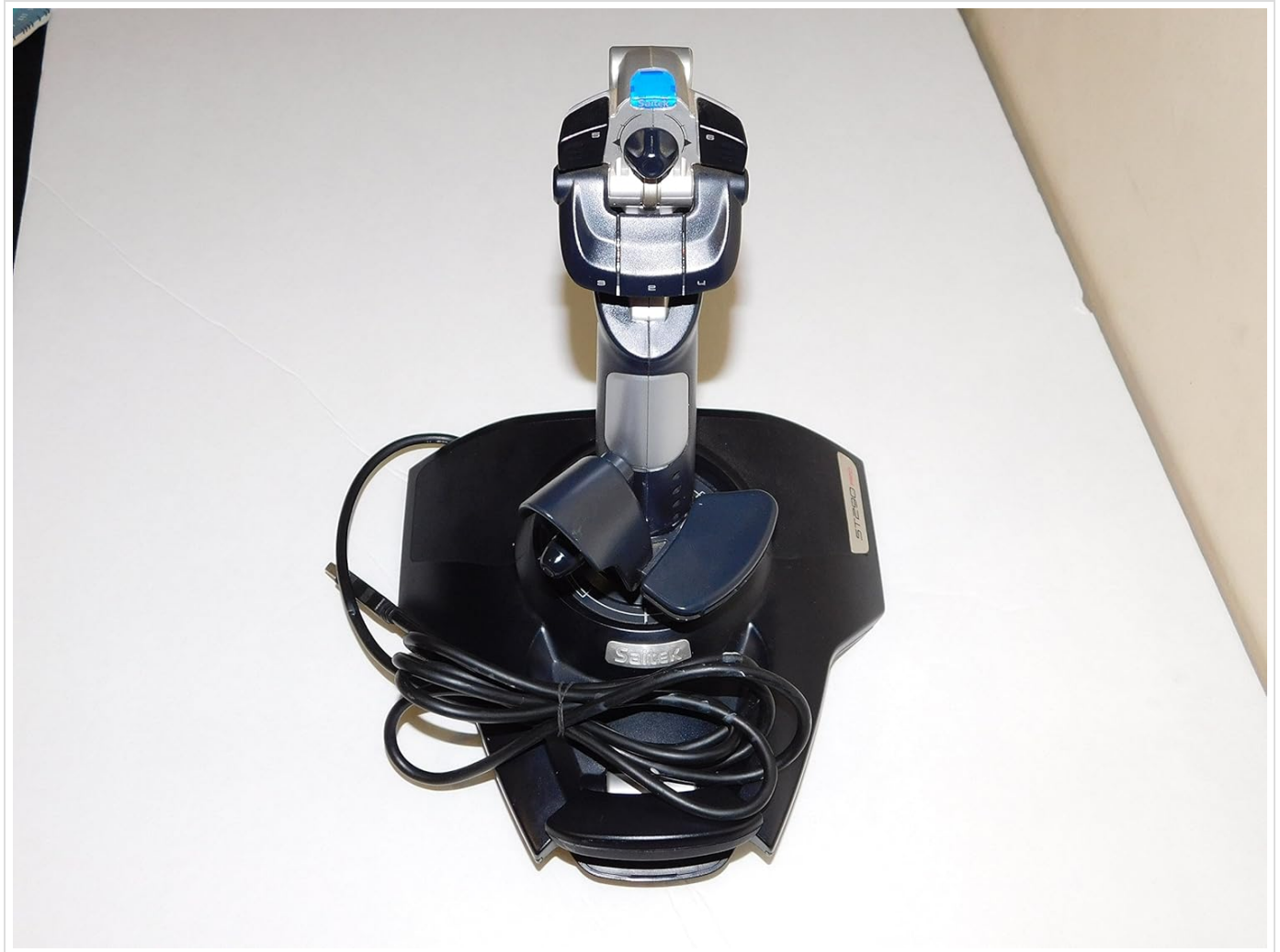
Front view of the Saitek ST290 Programmable Joystick, showing the main stick, base, and integrated throttle.
