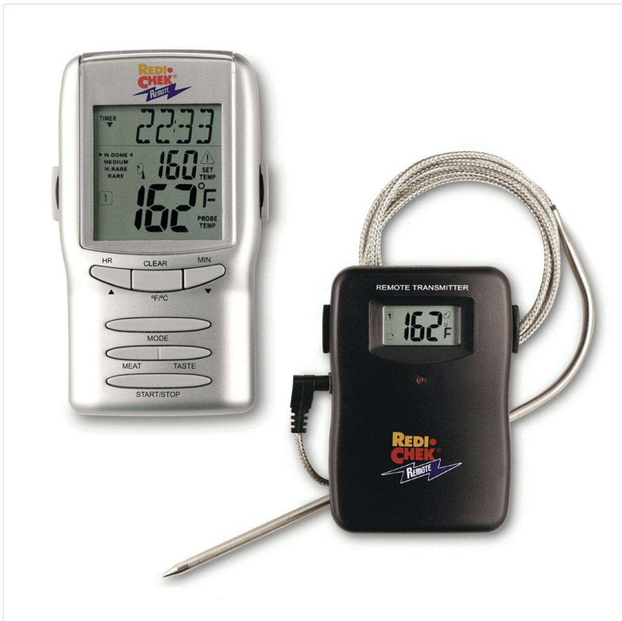
Image: The MAVERICK RediCheck ET-72 Remote Cooking Thermometer components, including the main receiver unit, the transmitter unit, and the stainless steel food probe with its heat-resistant wire.
