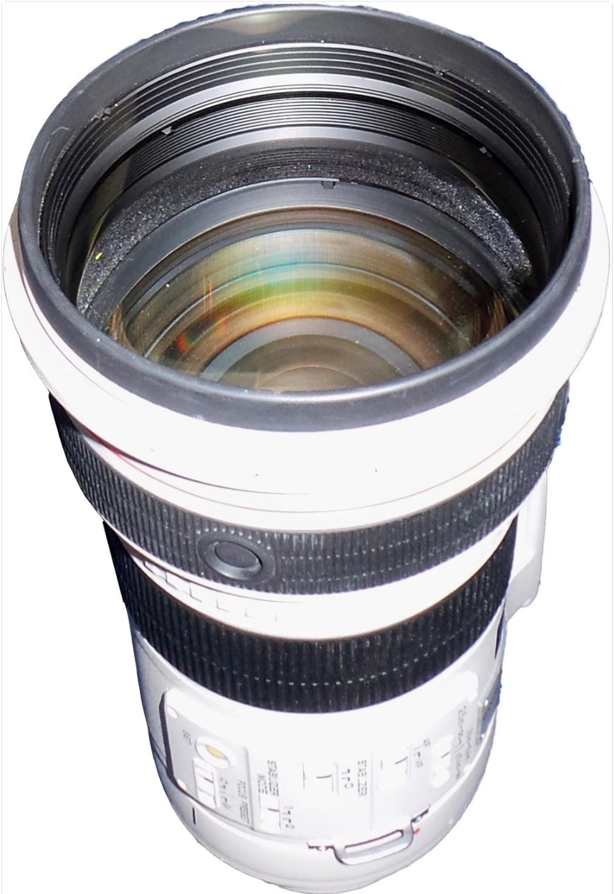
Figure 2: Front element of the lens, where the lens hood attaches.
