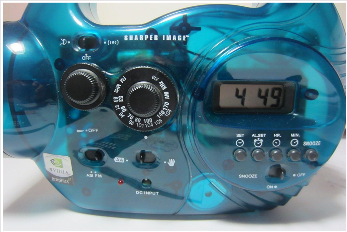
Figure 3: Detailed close-up of the control panel and LCD display on the Sharper Image YW631. This view shows the tuning knobs, function switches, and alarm clock buttons.
