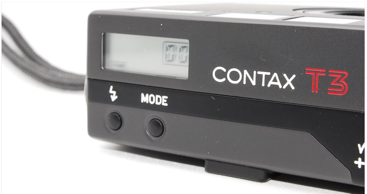
Figure 6: Display and Buttons. A close-up of the camera's top LCD display and adjacent control buttons, used for adjusting settings like flash mode and self-timer.
