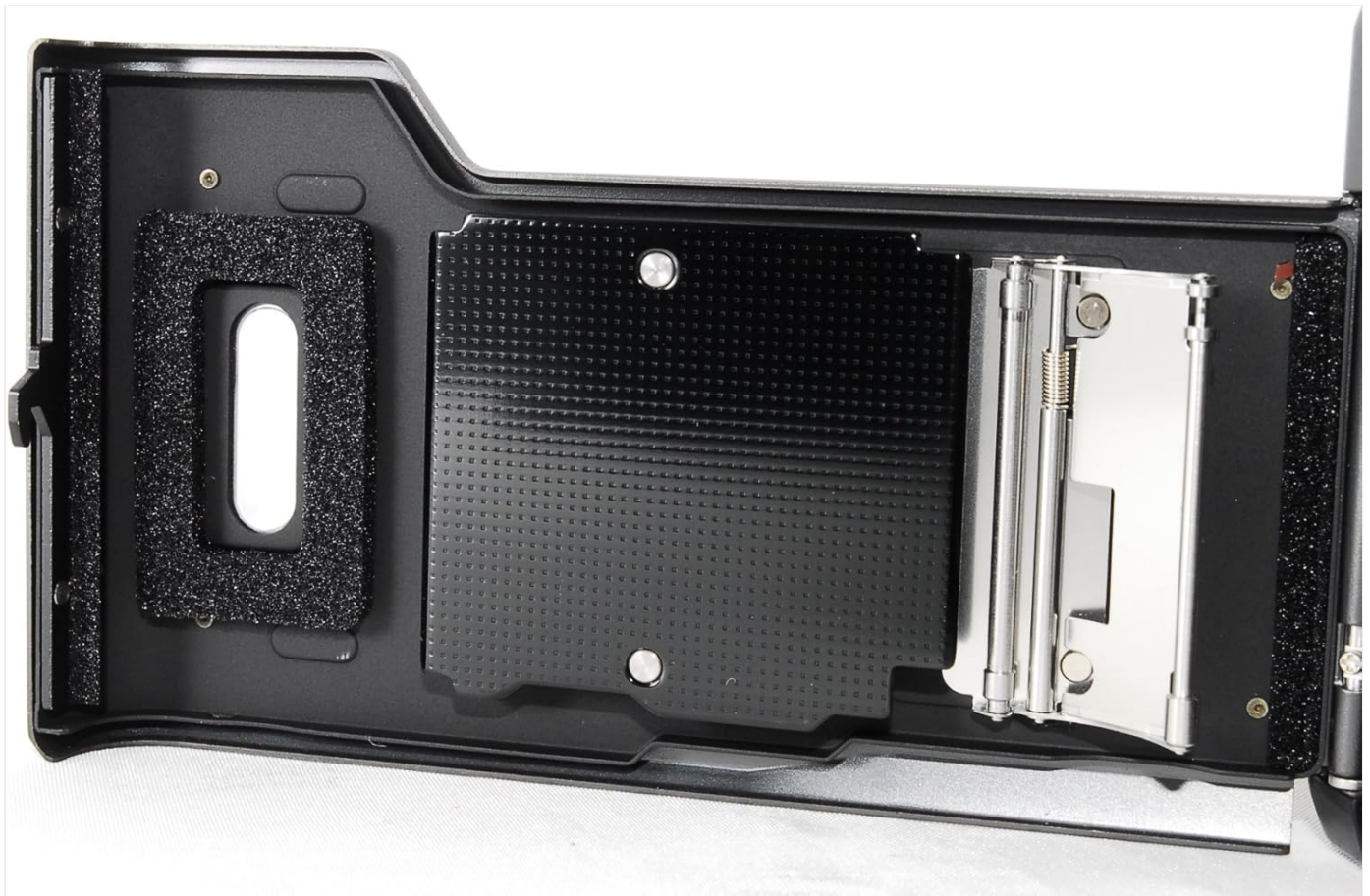
Figure 4: Film Compartment Interior. A detailed view of the film compartment, highlighting the film pressure plate and the mechanism for film advancement, crucial for proper film loading.
