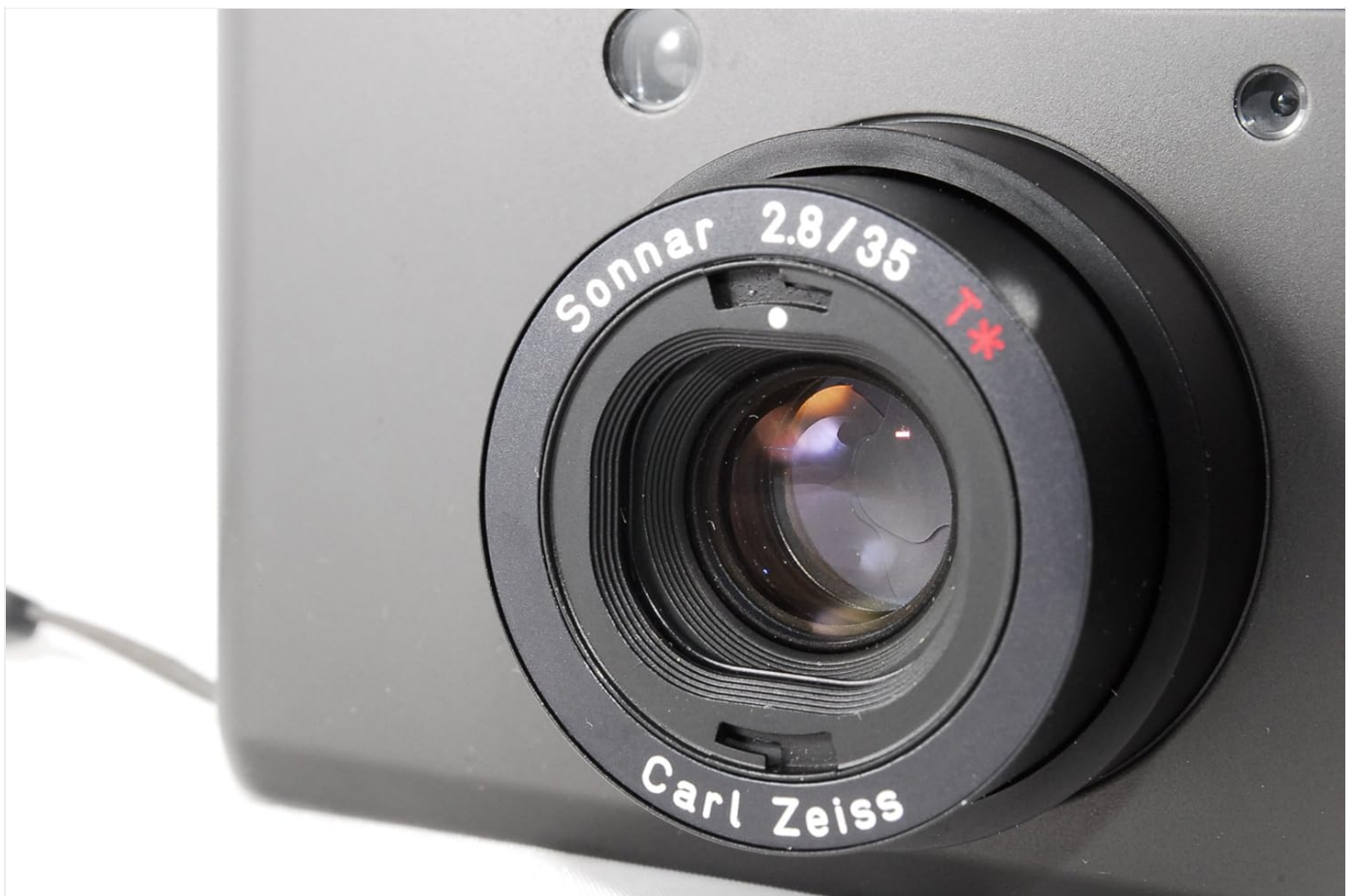
Figure 8: Lens Detail. A close-up view of the Carl Zeiss Sonnar 35mm f/2.8 lens, highlighting its markings and optical elements, which are central to the camera's image quality.
