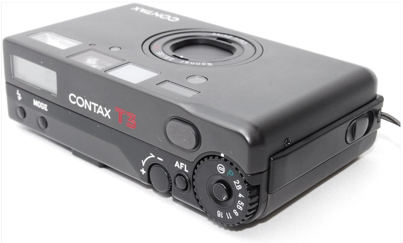
Figure 5: Top Controls. This image shows the top panel of the CONTAX T3, featuring the power switch, shutter release button, and the mode dial for various camera settings.
