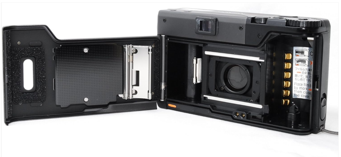
Figure 3: Open Film Compartment. This image displays the CONTAX T3 with its back cover open, showing the film chamber on the left and the take-up spool on the right, ready for film loading.
