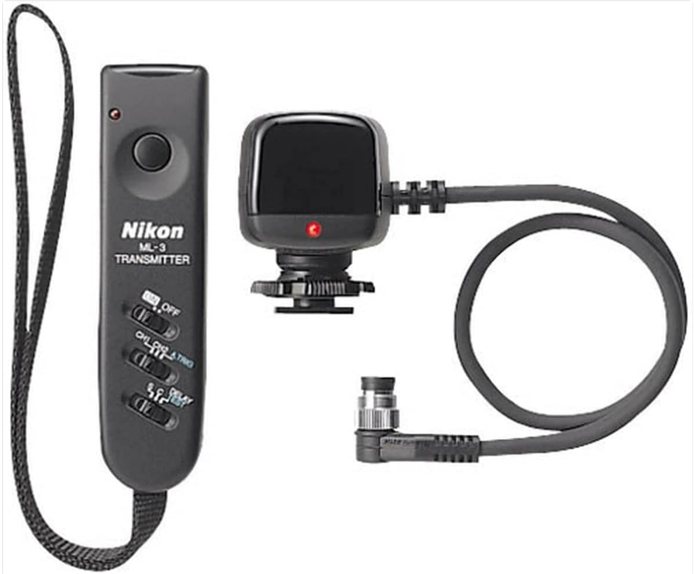
Figure 2: The Nikon ML-3 transmitter (left), receiver (top right), and connecting cable (bottom right). The receiver connects to the camera's 10-pin port, and the transmitter sends infrared signals to the receiver.
