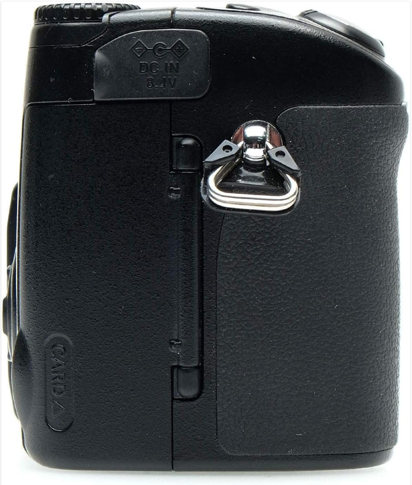
Image 3: Side View. This image illustrates the side of the Nikon Coolpix 5400, where the memory card compartment cover is located. Also visible is the DC IN port for connecting an optional AC adapter.
