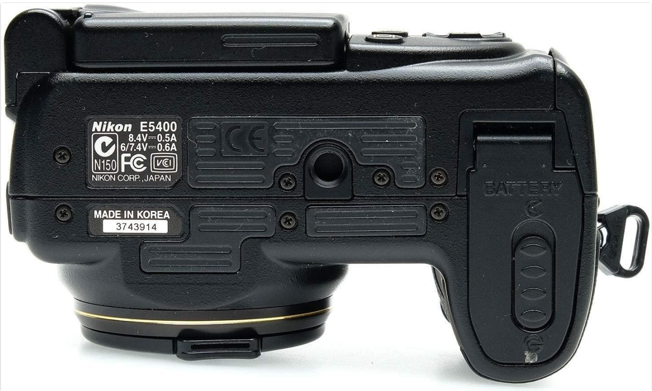
Image 4: Bottom View. This image displays the bottom of the Nikon Coolpix 5400, showing the battery compartment, the tripod mount thread, and regulatory information including the 'Made in Korea' label.
