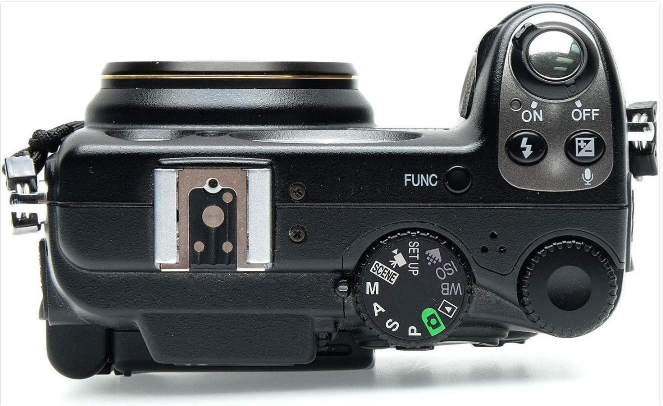
Image 2: Top View. This image shows the top panel of the Nikon Coolpix 5400, featuring the mode dial with various shooting settings (P, S, A, M, Scene, ISO, WB), the power on/off switch, the shutter release button, and a hot shoe for external flash units.
