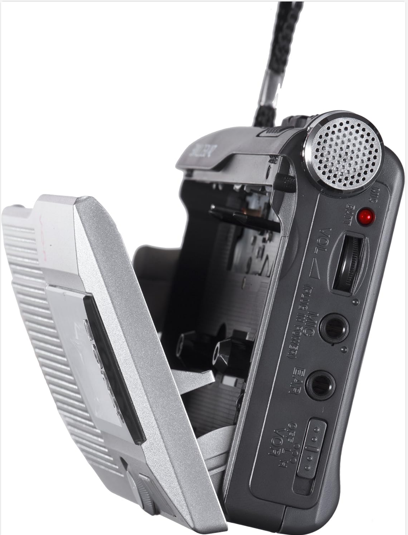
Figure 4.2: Side view of the Sony TCM-200DV with the cassette compartment door open, ready for tape insertion.
