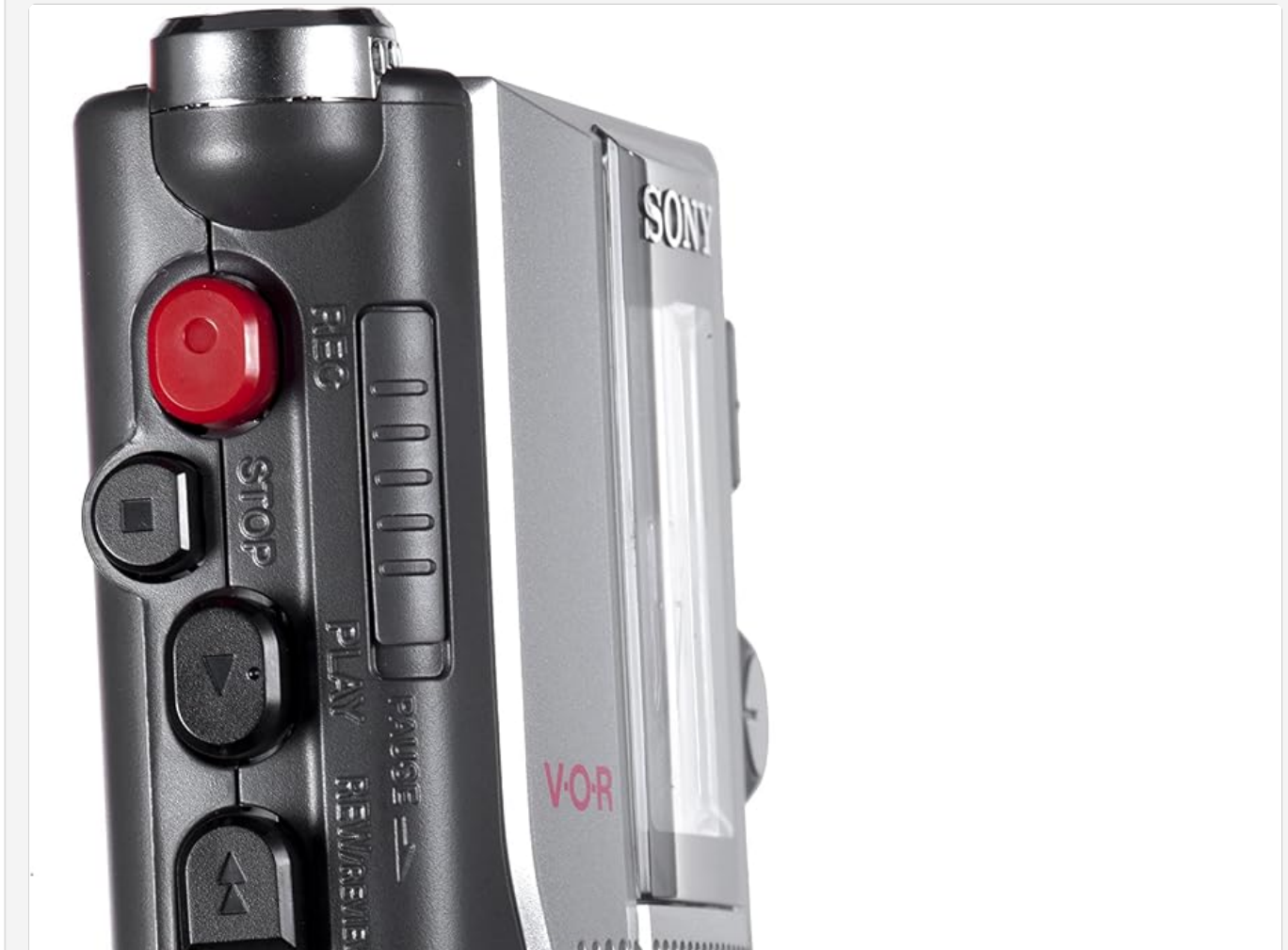
Figure 5.1: Front view of the Sony TCM-200DV, showing the speaker grille, cassette window, and main controls.
