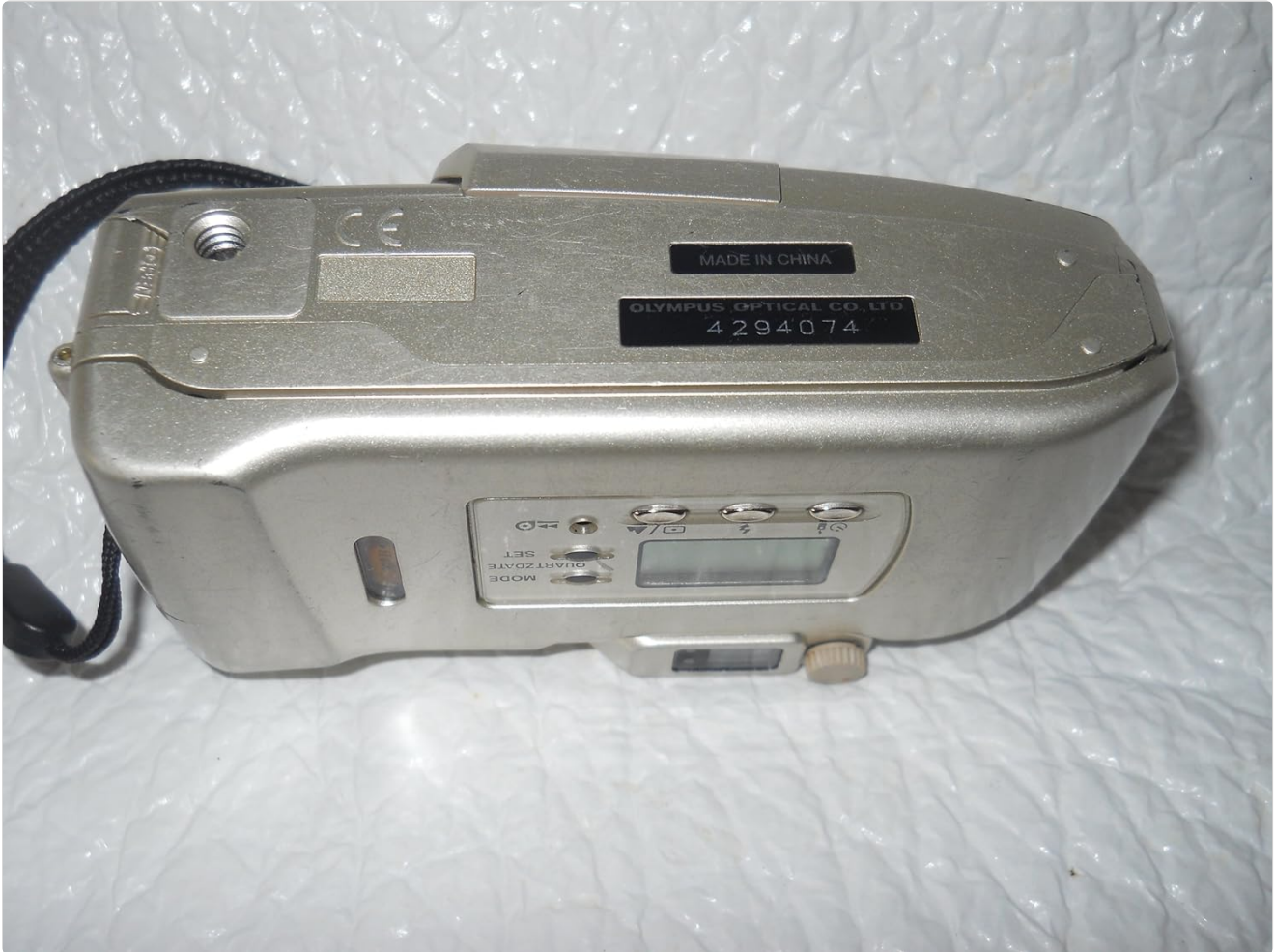
Figure 2: Bottom view of the camera, indicating the battery and film compartment area.
