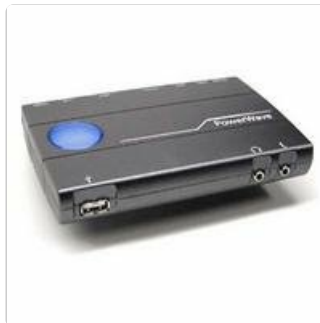
Figure 1: The Griffin PowerWave USB Audio Interface and Desktop Amplifier. This device connects to your computer via USB and provides various audio inputs and outputs.
