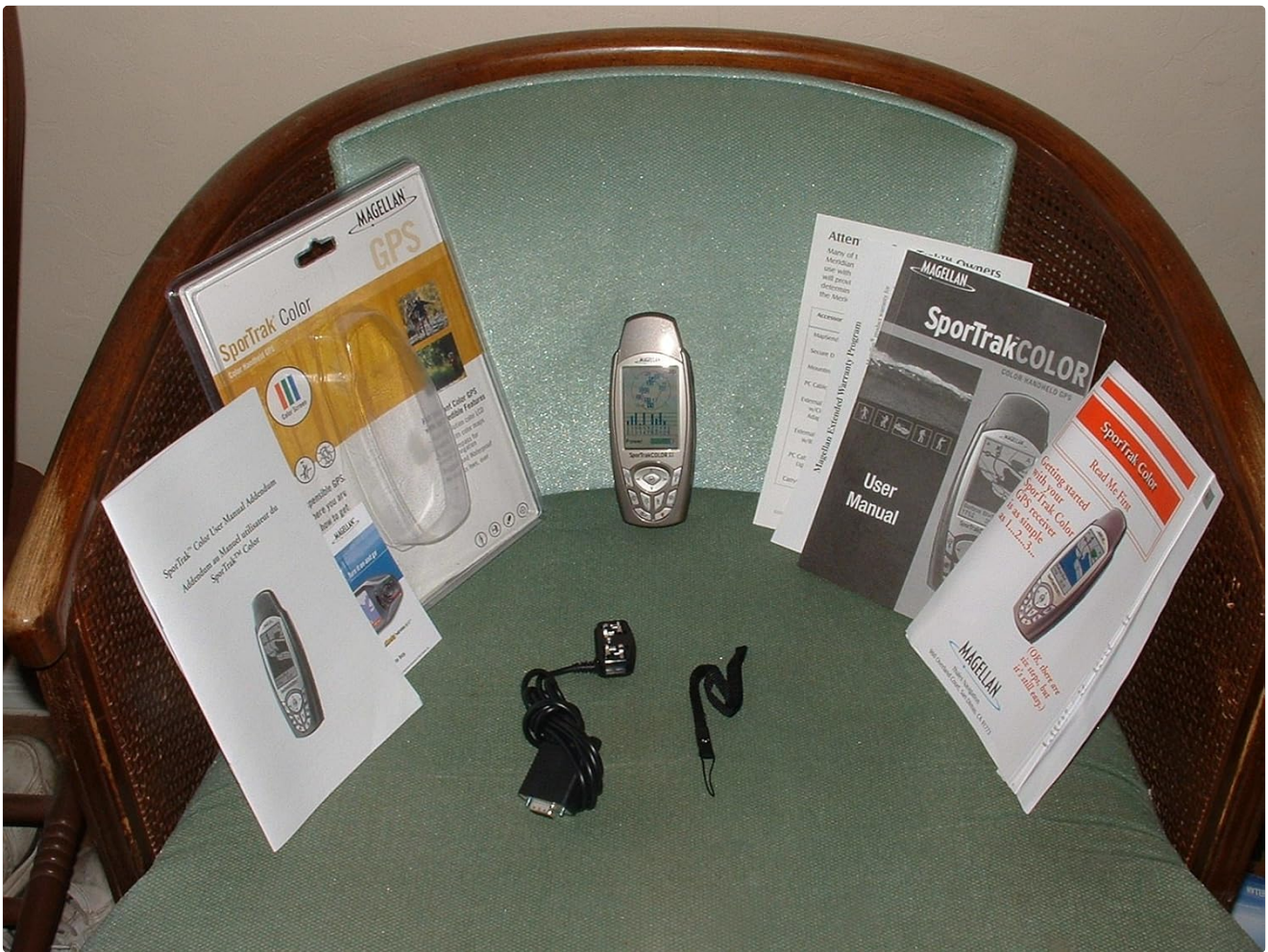
Figure 1: Contents of the Magellan SporTrak Color GPS packaging, showing the device, PC cable, manuals, and wrist strap.
