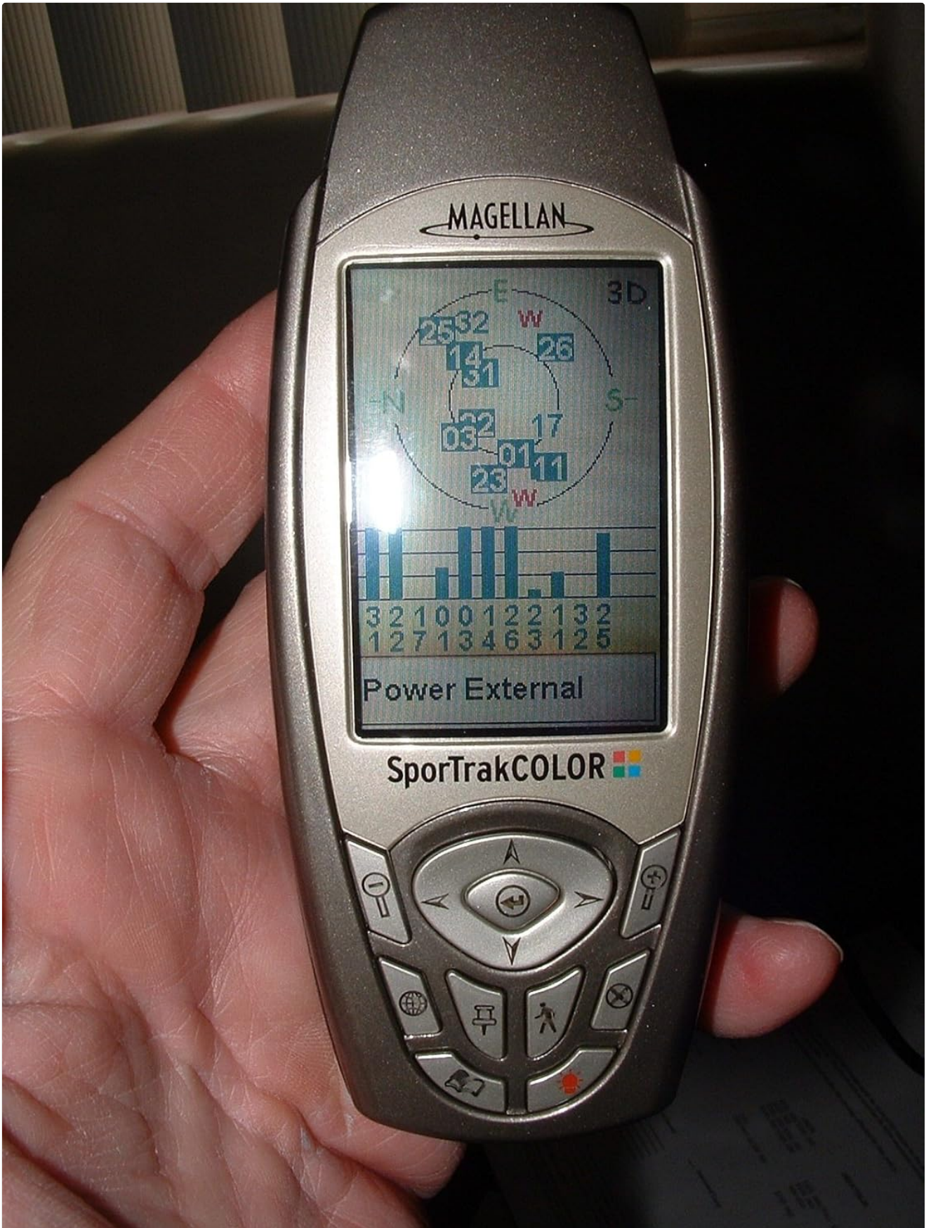
Figure 4: Device display showing satellite signal acquisition and power status.
