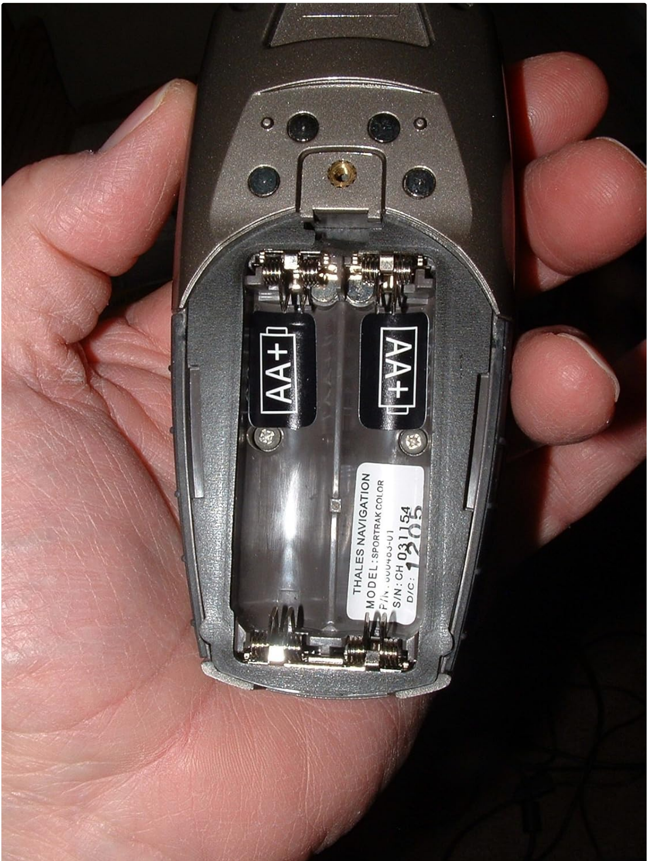
Figure 2: Battery compartment showing two AA batteries installed.
