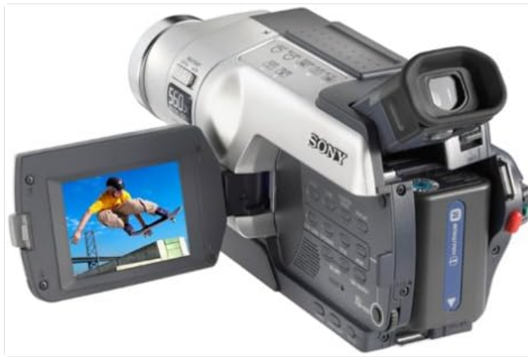
Figure 2.1: Rear view of the camcorder, showing the battery compartment and the open LCD screen.
