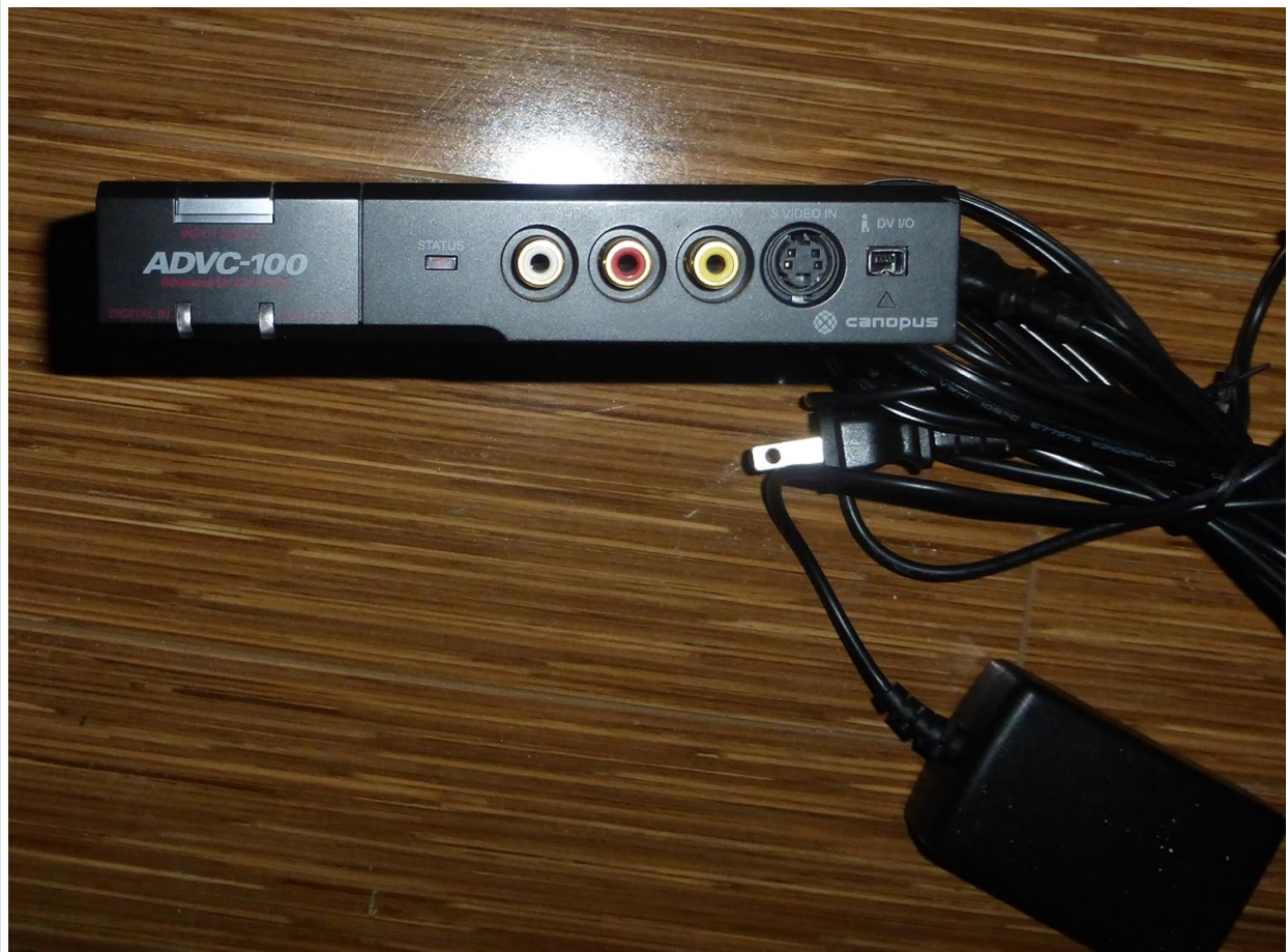
Figure 3.1: Front panel of the ADVC-100, featuring S-Video, Composite Video, and Audio (RCA) input jacks, along with a 4-pin DV (FireWire) port. This view highlights the primary connection points for analog video sources and a digital output to a computer.
