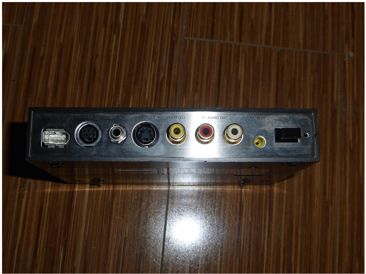
Figure 3.2: Rear panel of the ADVC-100, displaying analog output jacks (S-Video, Composite Video, Audio RCA), a 6-pin DV (FireWire) port, and the DC 5V power input. These ports are used for connecting to a display or for alternative digital output.
