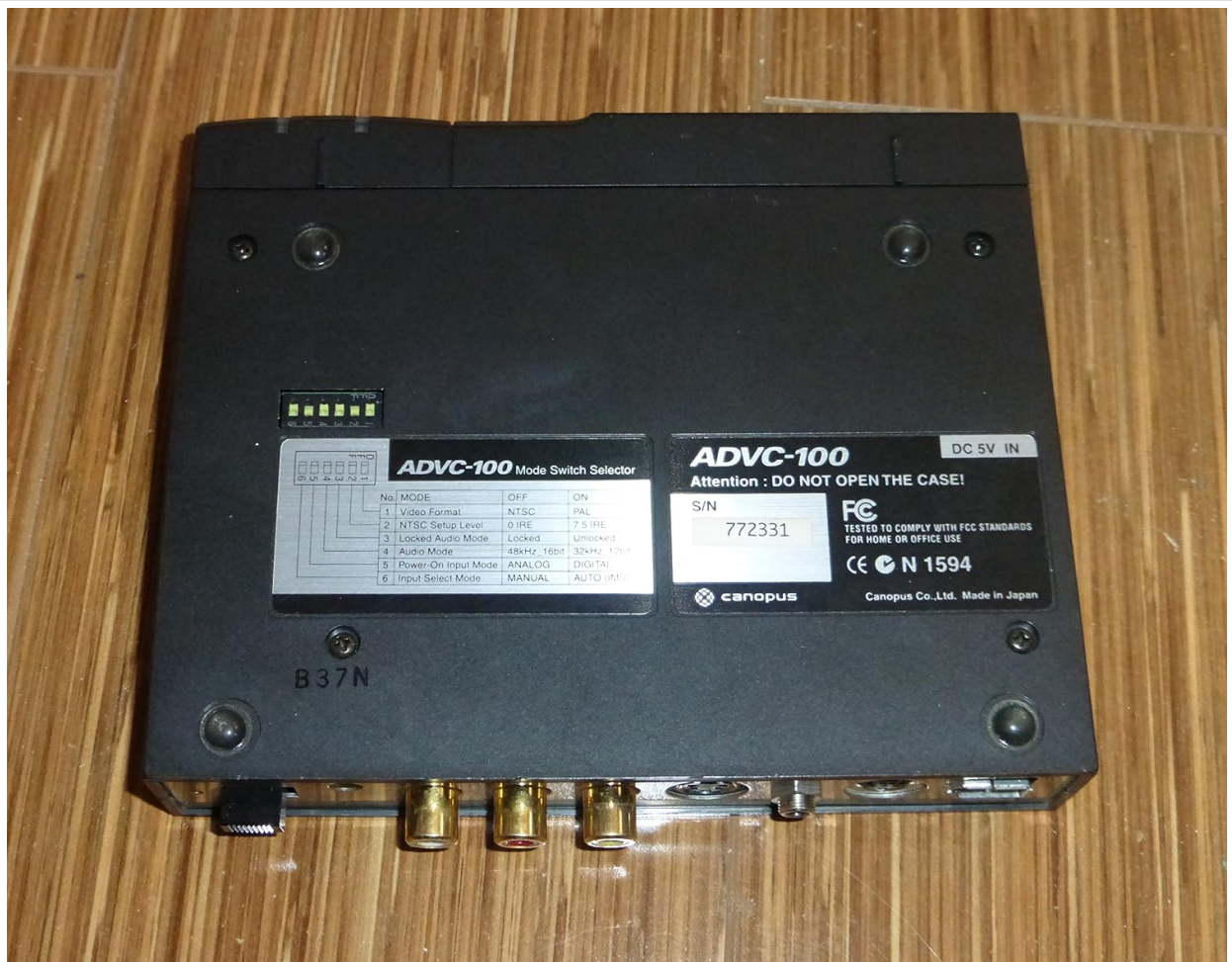
Figure 3.2: Rear panel of the ADVC-100, displaying analog output jacks (S-Video, Composite Video, Audio RCA), a 6-pin DV (FireWire) port, and the DC 5V power input. These ports are used for connecting to a display or for alternative digital output.
