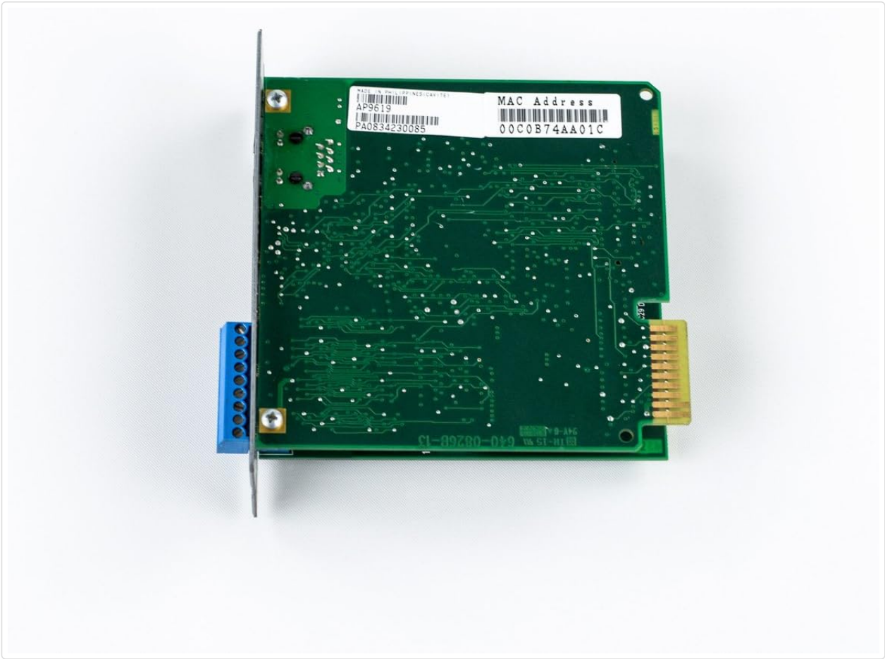
Figure 7.2: Rear view of the AP9619 card, displaying the product label with model and MAC address information.
