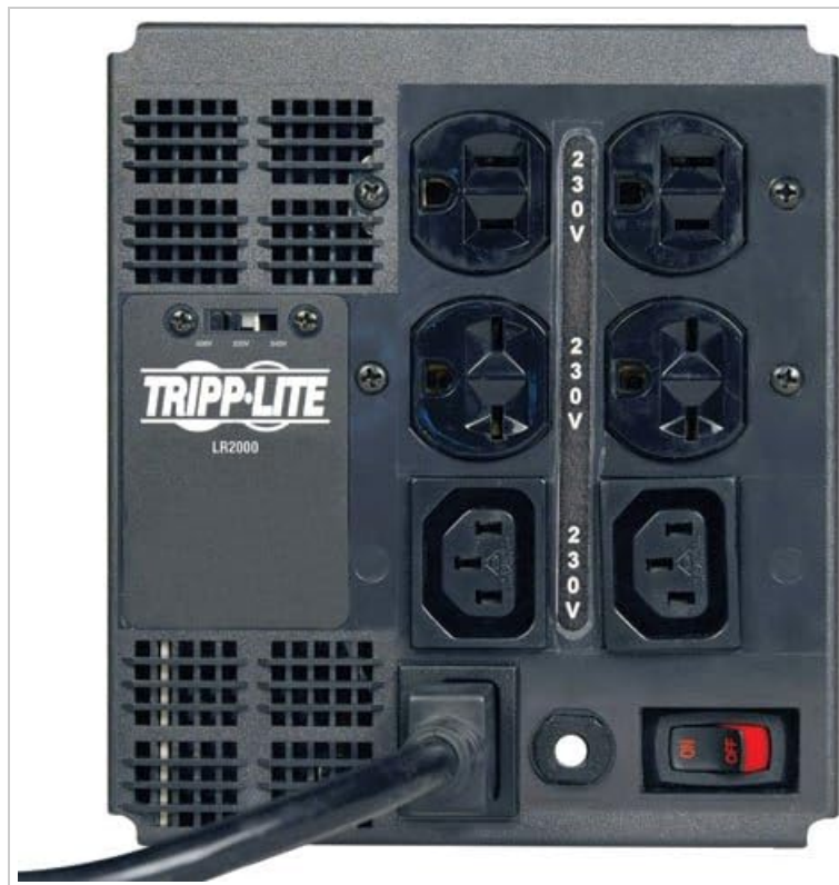
Figure 2: Rear view of the Tripp Lite LR2000 Line Conditioner, illustrating the six AC outlets (NEMA 5-15R, NEMA 6-15R, IEC-320) and the power switch.
