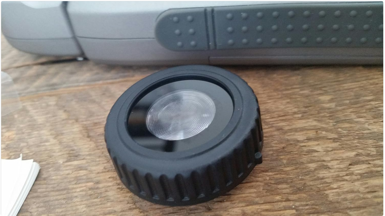
Image 3.3: The Lumigrid attachment for the Sekonic L-358. This accessory is used for reflected light measurements, focusing on light bouncing off the subject.
