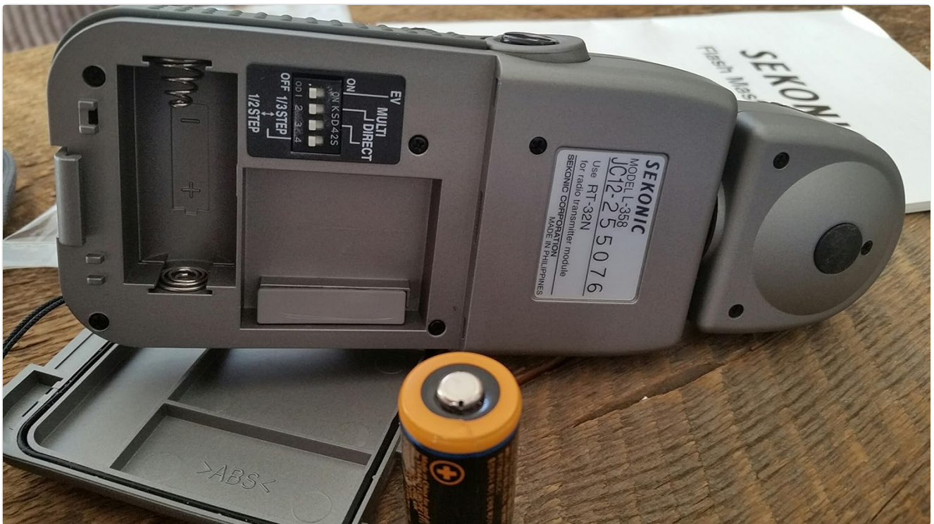
Image 3.2: Sekonic L-358 with the Lumisphere extended. This configuration is used for incident light measurements, capturing the light falling onto the subject.
