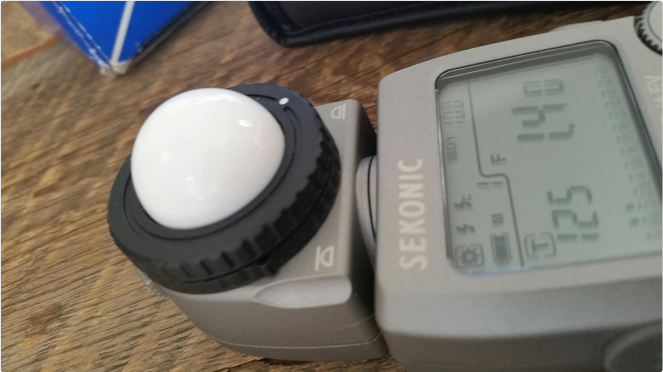
Image 3.4: Close-up of the Sekonic L-358 LCD display. This image illustrates how exposure values, ISO, and other settings are presented on the meter's screen during operation.
