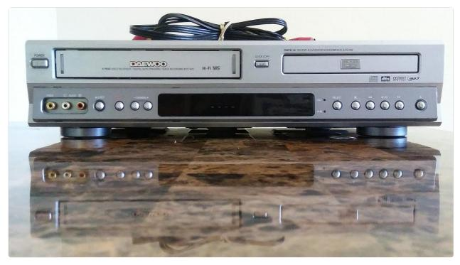
This image displays the front panel of the Daewoo DV6T811N DVD-VCR Combo. On the left, the VCR tape slot is visible with 'DAEWOO' branding and 'Hi-Fi VHS' label. To the right, the DVD tray is located. Below these, the control panel features buttons for power, video/audio inputs, eject, channel selection, quick copy, and DVD/VHS mode selection, along with standard playback controls (play, pause, stop, fast forward, rewind, skip). The display screen is centrally located.
