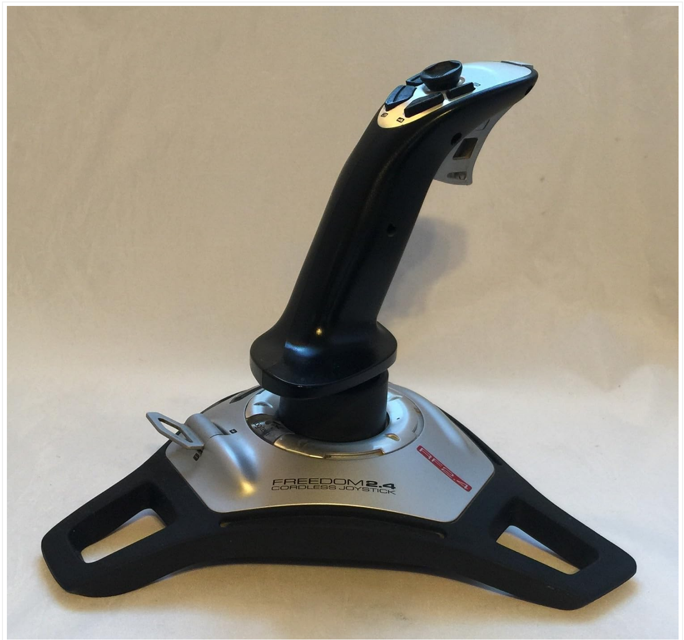
Figure 1.1: Front view of the Logitech G Freedom 2.4 GHz Cordless Joystick, showcasing its ergonomic design and button layout.
