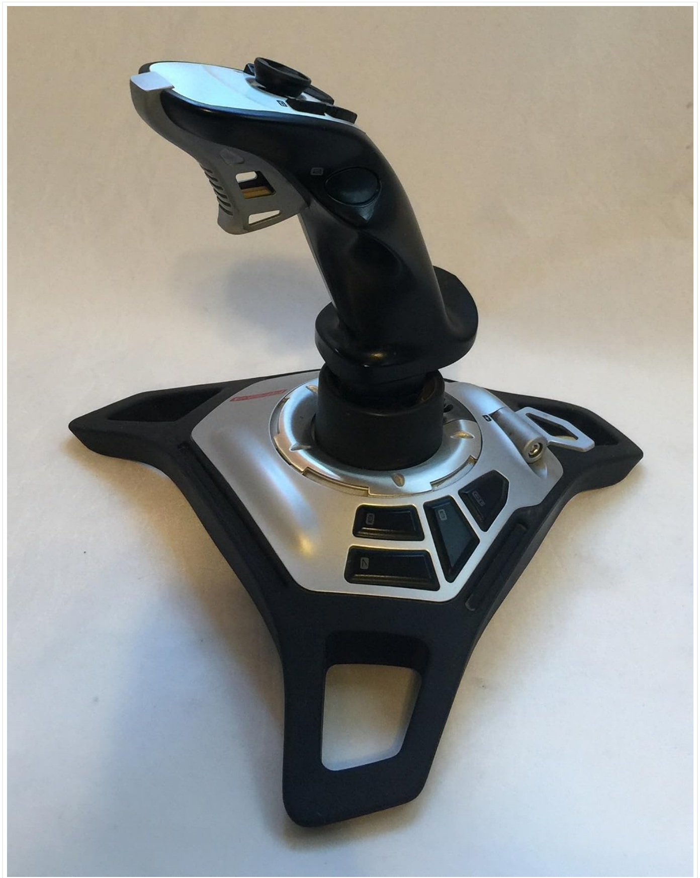
Figure 3.1: Side view of the joystick, highlighting the placement of the programmable buttons and the throttle lever.
