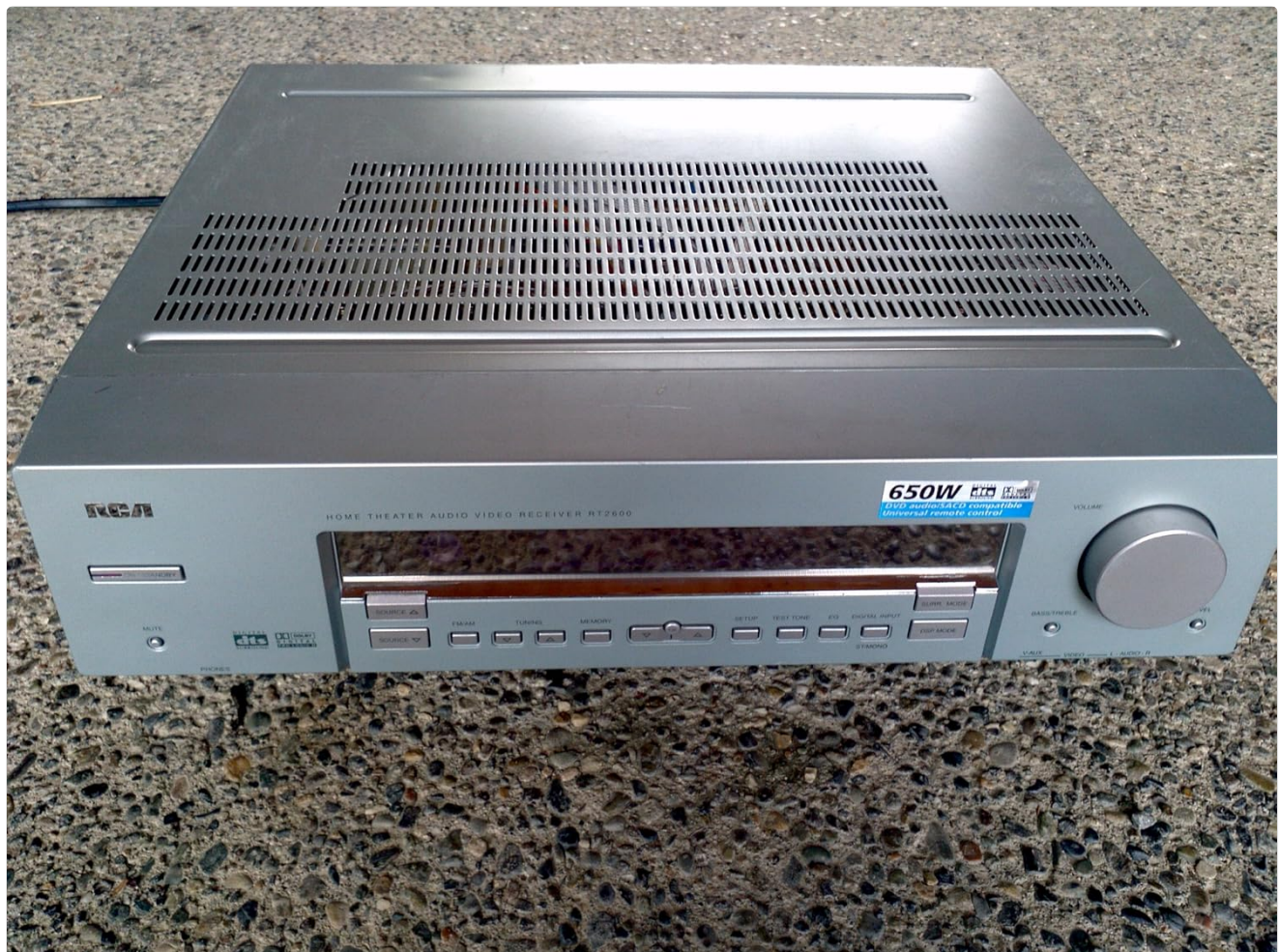
Figure 4.1: The RCA RT2600 Home Theater Audio Video Receiver. This silver unit features a central display, various control buttons for functions like tuning, memory, setup, and input selection, and a large volume knob on the right. The top surface has ventilation
