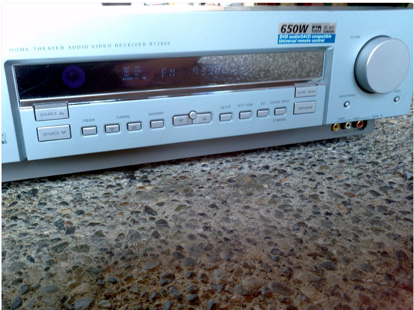
Figure 5.1: A close-up view of the RCA RT2600 receiver's front panel, highlighting the display showing "FM 93.9MHz" and various control buttons. These include "SOURCE A" and "SOURCE V" for input selection, "FM/AM", "TUNING", "MEMORY", "SETUP", "TEST TONE", "EQ", "DIGITAL INPUT", and "DSP MODE" buttons. A large volume knob is visible on the right.
