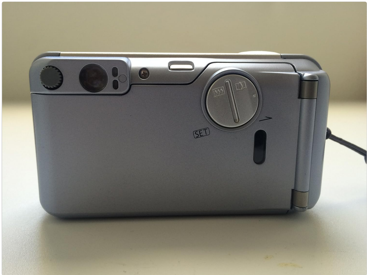
Figure 6.1: Back view of the Canon Sure Shot 130u camera. This image shows the film compartment door, the film advance/rewind mechanism, and other rear controls.
