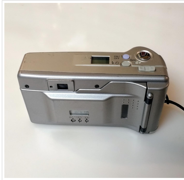
Image: Top view of the Minolta Zoom 80 camera, indicating the ON/OFF switch and zoom controls.
