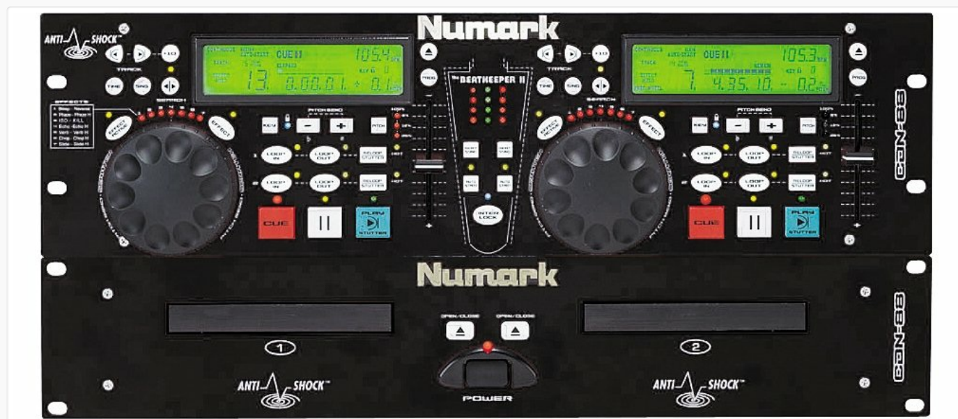
Figure 4.1: Front view of the Numark CDN88 PRO Dual CD Player, showing the control unit positioned above the drive unit.
