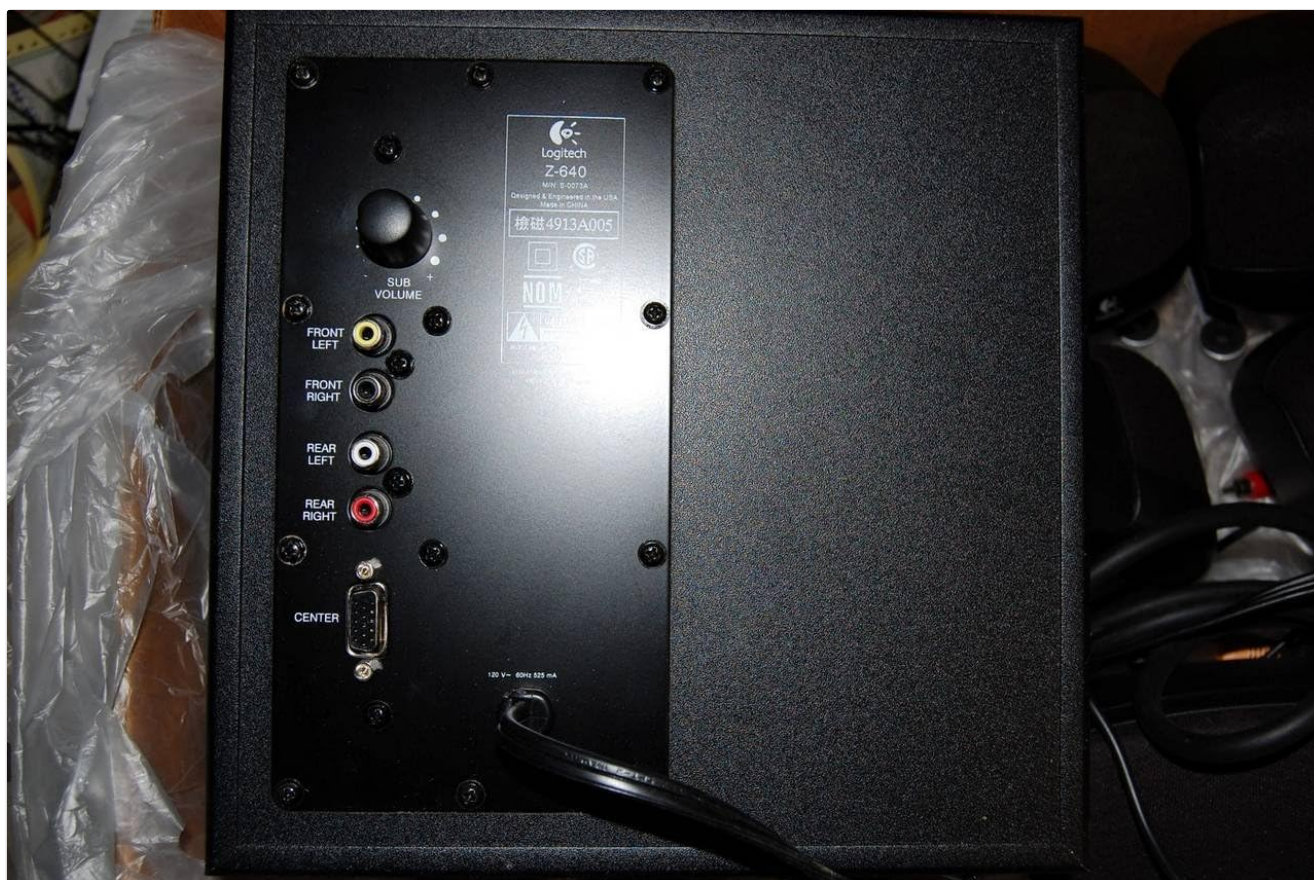
Image: Rear panel of the Logitech Z-640 subwoofer, showing the color-coded input jacks for front, rear, and center/subwoofer channels, along with the sub volume knob and power cable.
