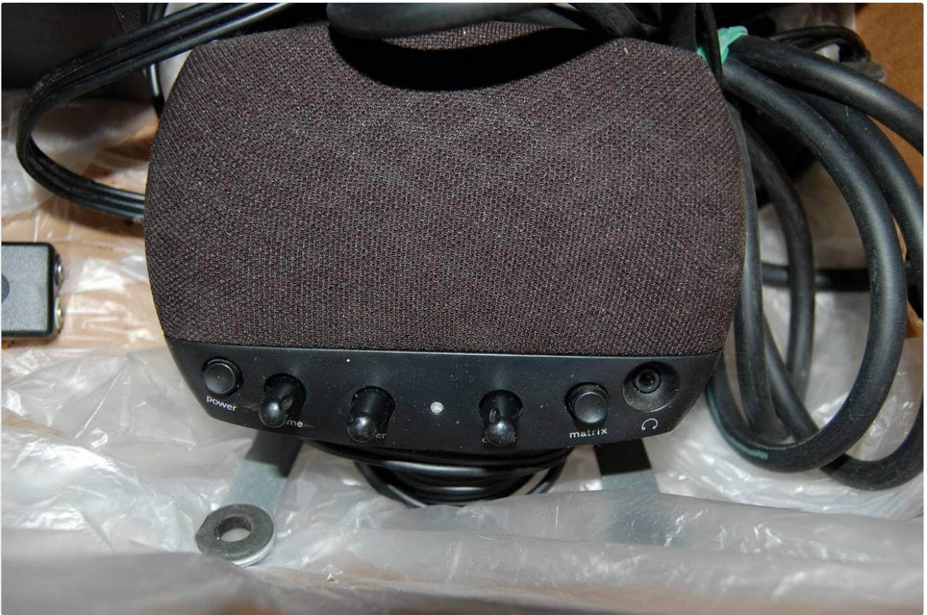
Image: Close-up of the Logitech Z-640 center speaker, displaying the control panel with buttons for power, volume, matrix mode, fader, and a headphone jack.
