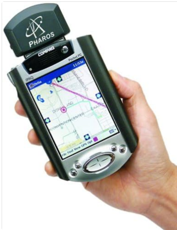
Figure 2.1: The PHAROS PF022 CompactFlash GPS receiver inserted into the top slot of a Pocket PC device. The Pocket PC screen displays a map with a highlighted route and navigation information, indicating the device's primary function as a portable navigation system. A hand is holding the Pocket PC.
