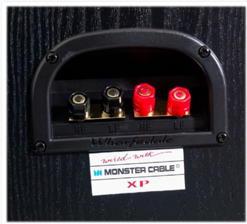
Figure 3: Close-up view of the dual gold-plated speaker terminals on the rear of the Wharfedale Diamond 8.4, showing connections for bi-wiring/bi-amping.
