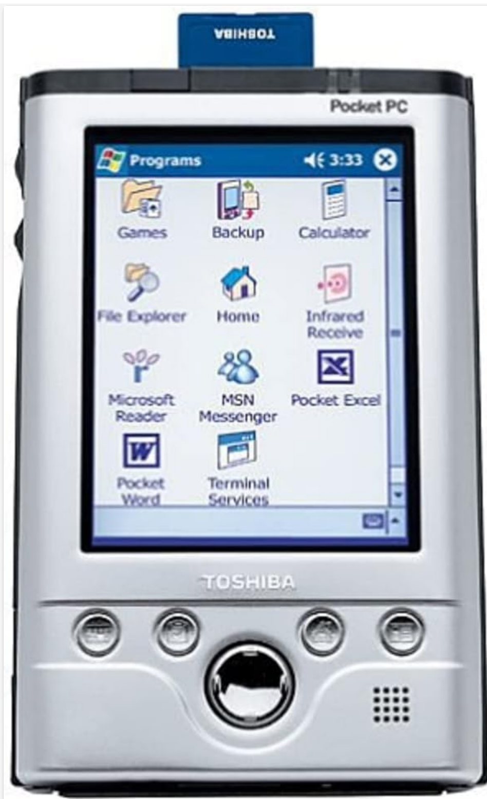
Figure 1: Toshiba e740 Pocket PC. This image shows the Toshiba e740 Pocket PC, a compact handheld device. The screen displays a grid of application icons including 'Programs', 'Games', 'Backup', 'Calculator', 'File Explorer', 'Home', 'Infrared Receive', 'Microsoft Reader', 'MSN Messenger', 'Pocket Excel', 'Pocket Word', and 'Terminal Services'. Below the screen, the 'TOSHIBA' logo is visible, along with four circular buttons and a central navigation pad. A blue Toshiba-branded card is partially visible inserted at the top of the device.
