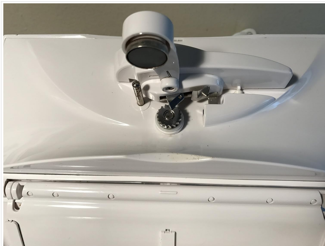
Figure 2: The can opening mechanism, visible when the front cover is pulled down. It features a cutting blade, guide wheel, and a magnet to secure the lid.
