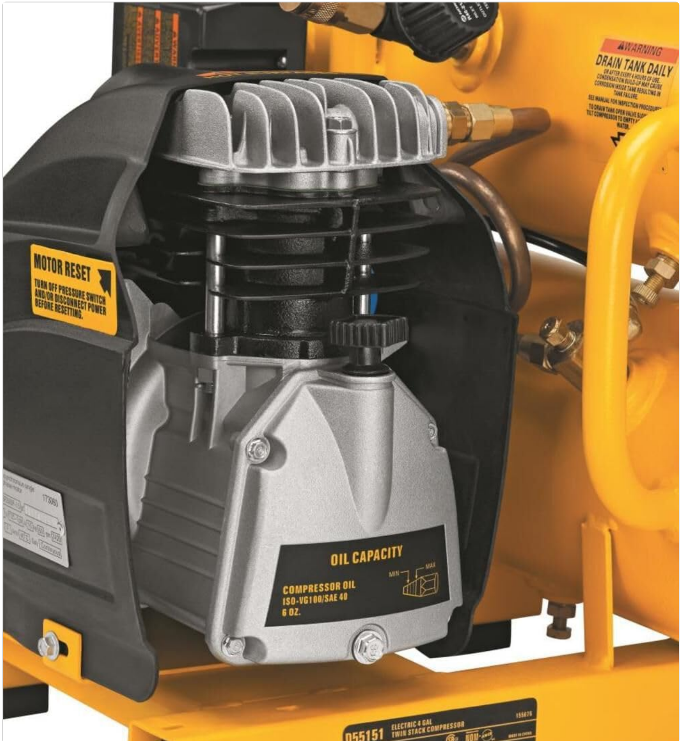
Figure 6.1: Location of the motor reset button on the DeWalt D55151. Press this button after the motor has cooled if it stops due to overload.
