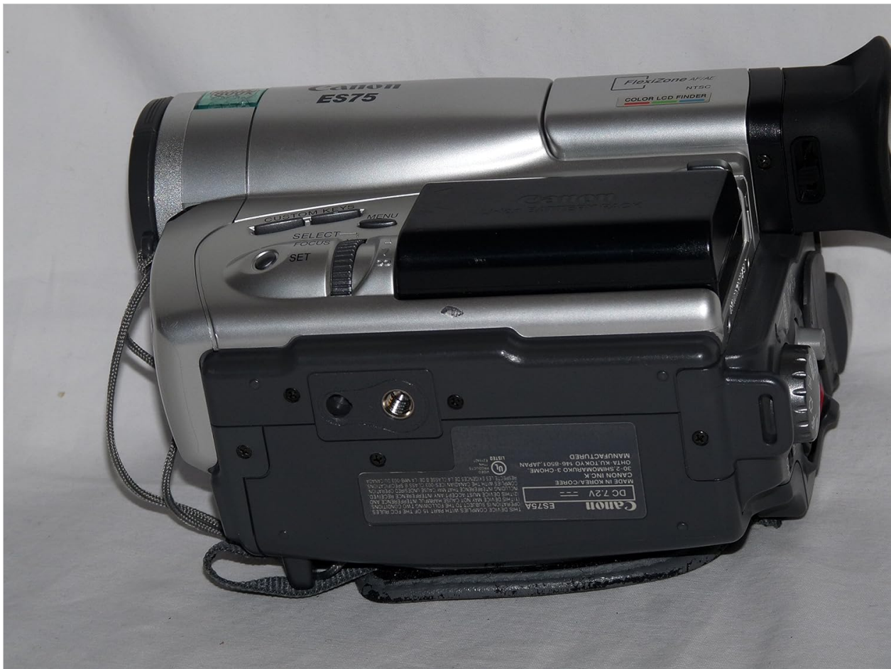
Figure 2: Battery compartment location on the Canon ES75.
