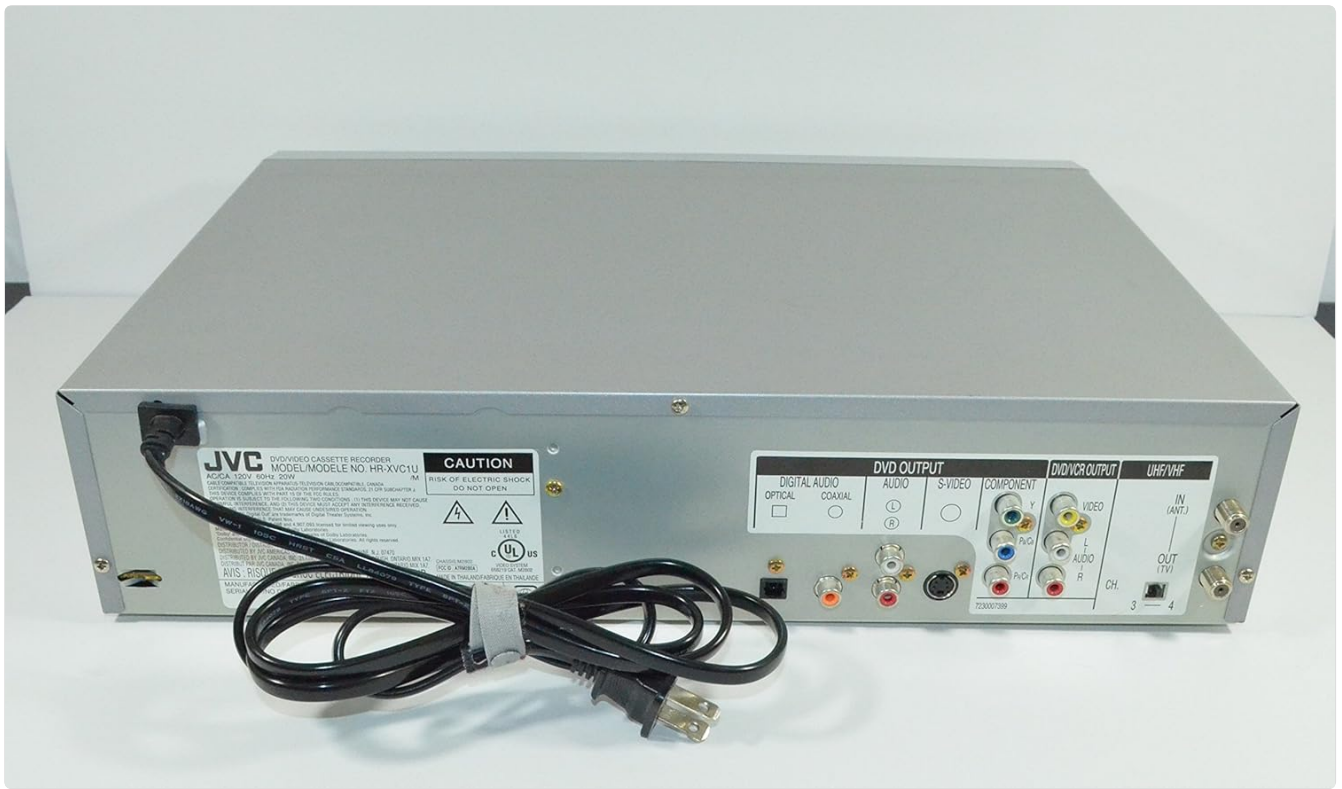
Image: The rear panel of the JVC HR-XVC1U, displaying the various connection ports including digital audio (optical, coaxial), S-video, component video, composite video, and RF input/output.
