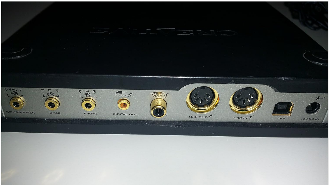
Image: The rear panel of the Sound Blaster Extigy, illustrating the various input and output ports including USB, MIDI, and analog/digital audio connections.
