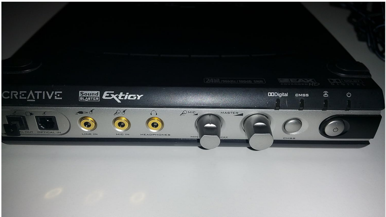
Image: The front panel of the Sound Blaster Extigy, detailing the Line In, Mic In, Headphone jacks, Master volume, Mic volume, CMSS button, and Power button.
