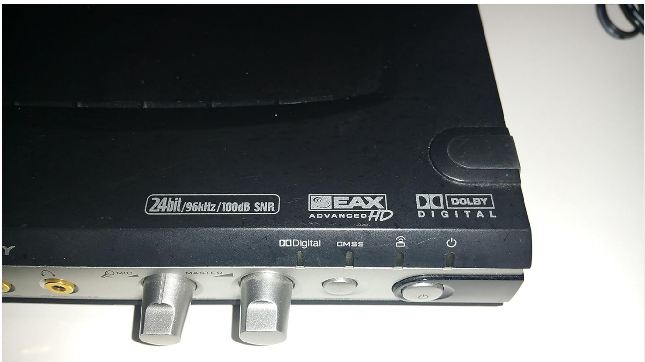
Image: A close-up view of the Sound Blaster Extigy's front panel, highlighting the 24-bit/96kHz/100dB SNR, EAX Advanced HD, and Dolby Digital branding, indicating its audio capabilities.
