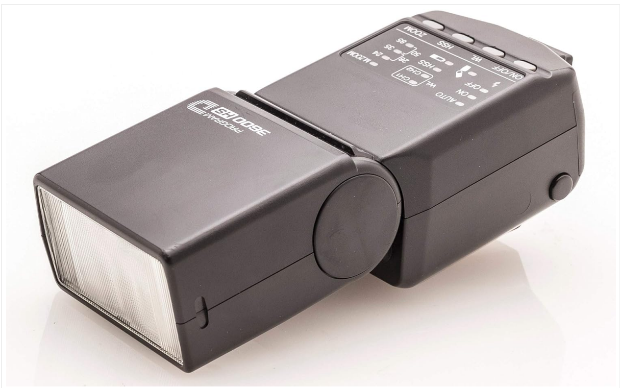
Figure 3.2: Top Control Panel. This image displays the top of the flash head, highlighting the control panel with buttons for ZOOM, HSS (High-Speed Sync), WL (Wireless), and the ON/OFF switch. Various indicators for flash modes (AUTO, M.ZOOM) and channels (CH1, CH2) are also visible.
